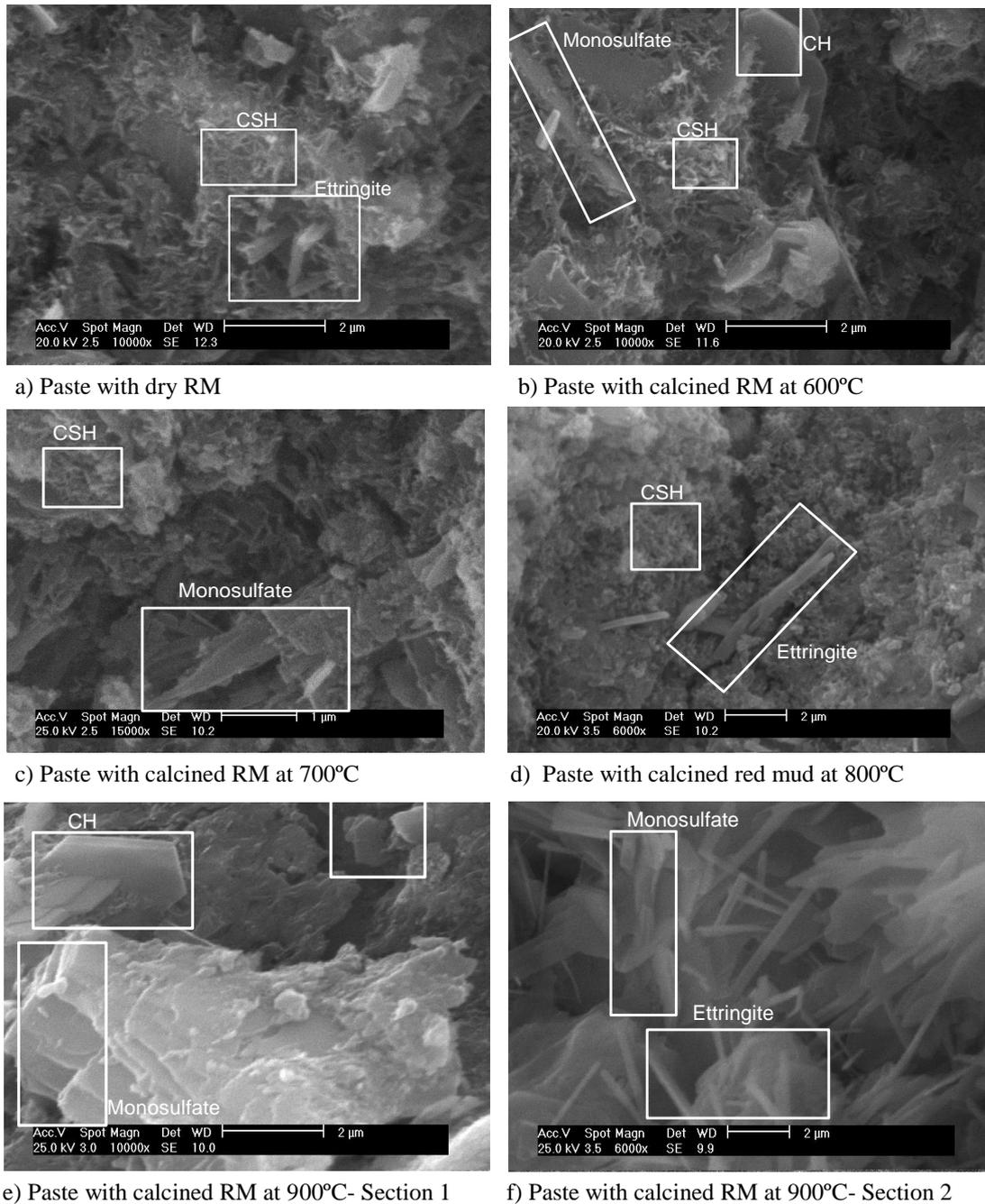
**Figure 4. Images of the microstructure of the pastes produced with 15% of RM at 28 days**
