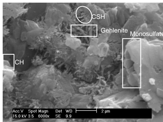
**Figure 3. Image of the microstructure of the reference paste at 28 days**
