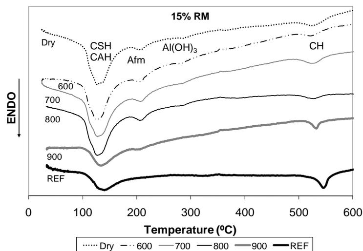
**Figure 2. Thermograms of the pastes produced with 15% of red mud and of the reference paste**
