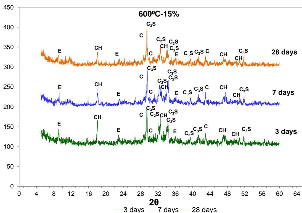
**Figure 1. Diffractograms of the pastes with 15% of red mud calcined at 600°C**
