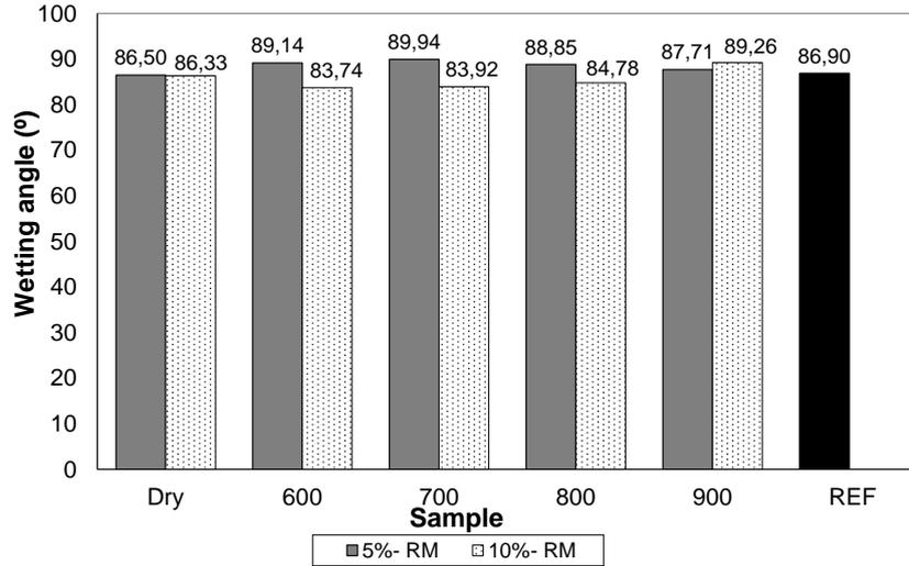
**Figure 8. Apparent wetting angle of the mortars**
