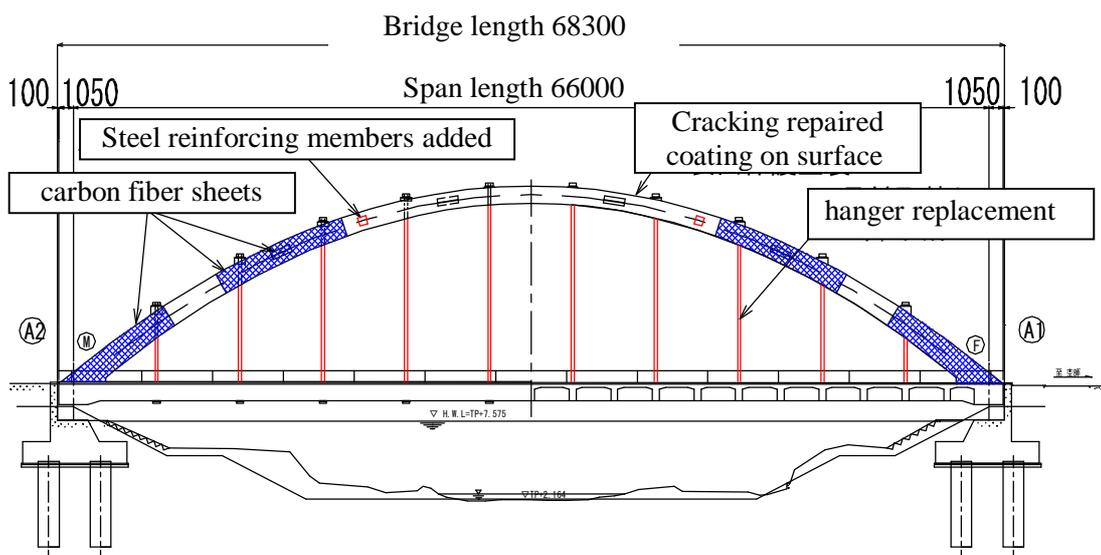
Figure 4. Outline of permanent repairs
