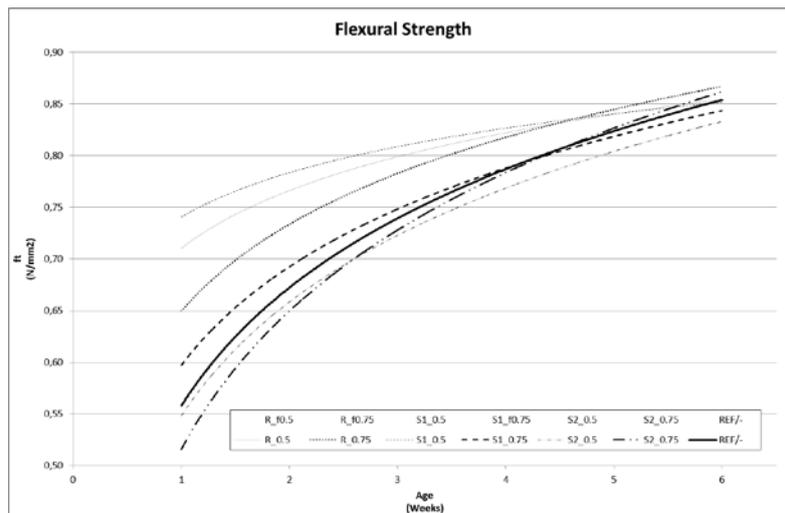
**Figure 3. Flexural Strength development**
