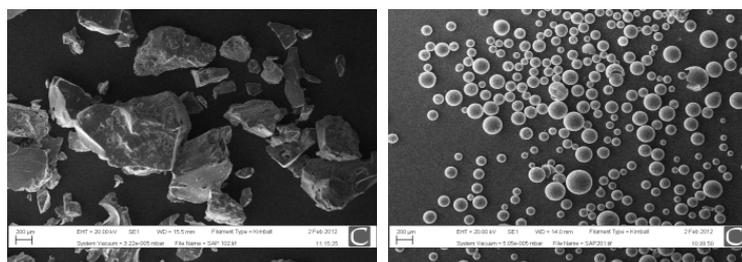
**Figure 1. Superabsorbent polymers, SAP 1 (left) and SAP 2 (right)**
