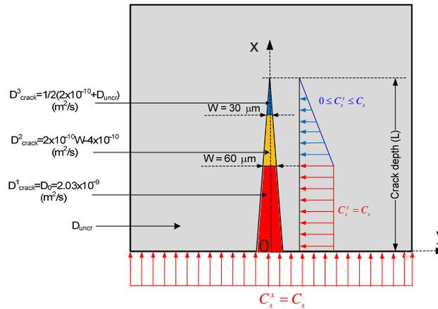
**Figure 12. The concept of the 2D surface content and diffusion coefficient of chloride for cracked concrete**
