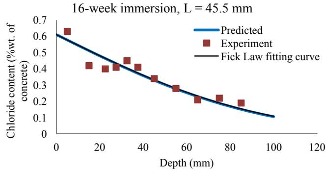
**Figure 11. Comparison between predicted and experimental results (W/C =0.5).**
