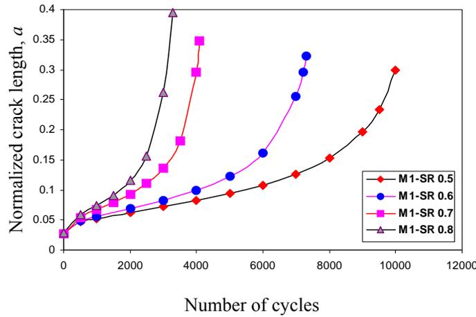
**Figure 2. Predictions of relationships of crack length and number of cycles**
