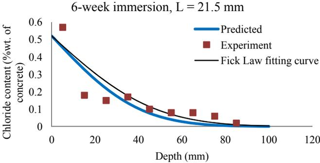
**Figure 9. Comparison between predicted and experimental results (W/C = 0.4).**
