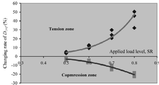
**Figure 4. The effect of applied load levels on chloride diffusion coefficient of concrete both in tension and compression**
