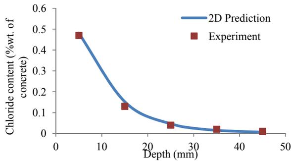
**Figure 15. The predicted and experimental results at 41mm away from crack plane.**
