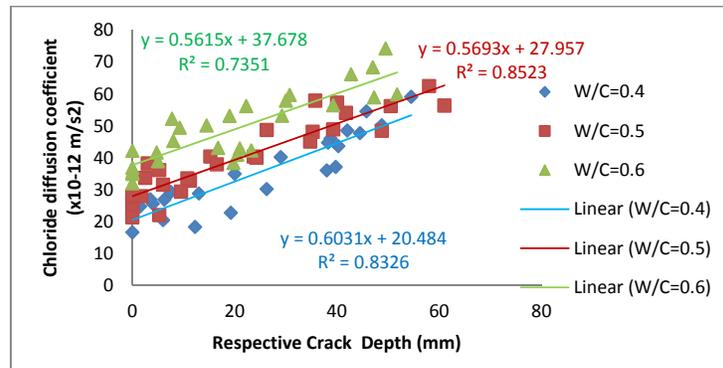
**Figure 7. The influence of crack depth on the chloride diffusion coefficient**
