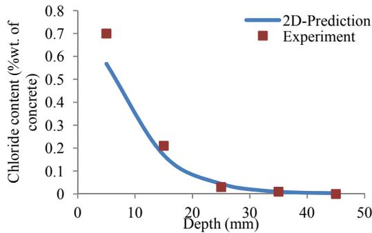
**Figure 16. The predicted and experimental results at 50mm away from crack plane.**
