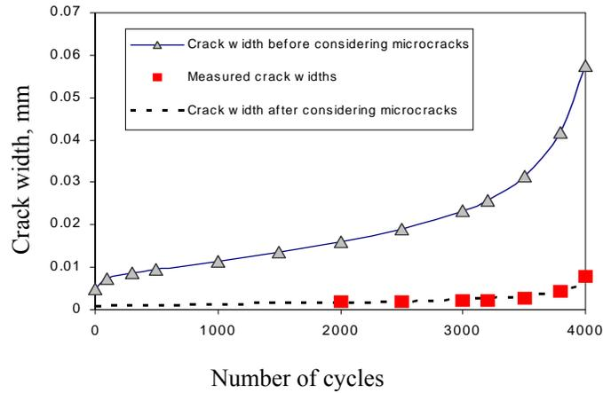
**Figure 3. Relationships of crack width and number of cycles, model prediction and experimental results,  $SR=0.7$**
