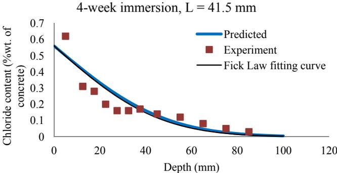
**Figure 8. Comparison between predicted and experimental results (W/C = 0.6).**
