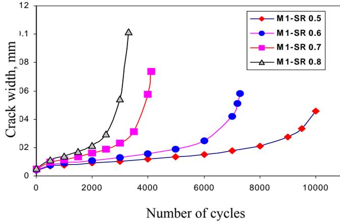
**Figure 1. Predictions of relationships of crack width and number of cycles**
