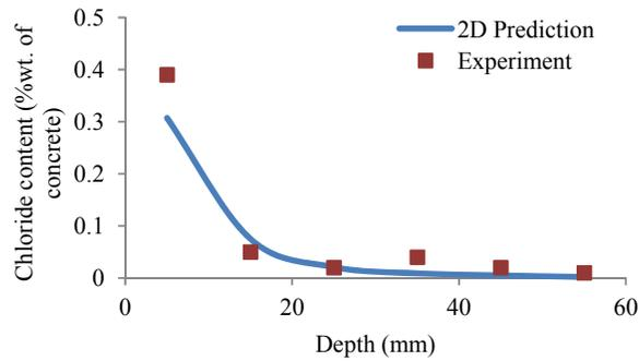
**Figure 14. The predicted and experimental results at 30mm away from crack plane**
