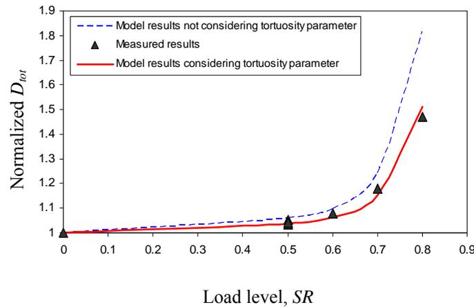
**Figure 5. Relationships of load level and normalized  $D_{tot}$ , model prediction and experimental results,  $N=3500$**
