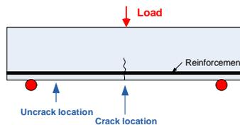
**Figure 6. Definition for crack and uncrack locations.**
