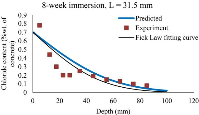
**Figure 10. Comparison between predicted and experimental results (W/C = 0.5).**
