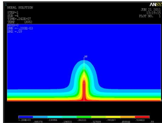
**Figure 13. The 2D chloride diffusivity model of cracked concrete beam 1**
