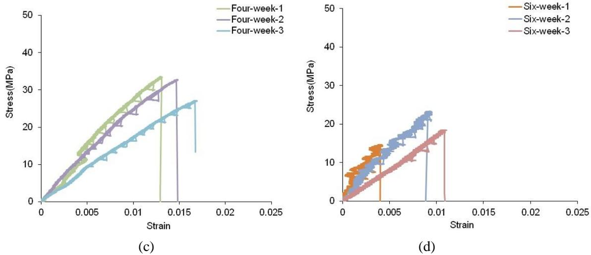
**Figure 7. Stress-strain behavior of epoxy exposed to sulfuric acid: (a) 0 week; (b) 2 weeks; (c) 4 weeks; (d) 6 weeks**
