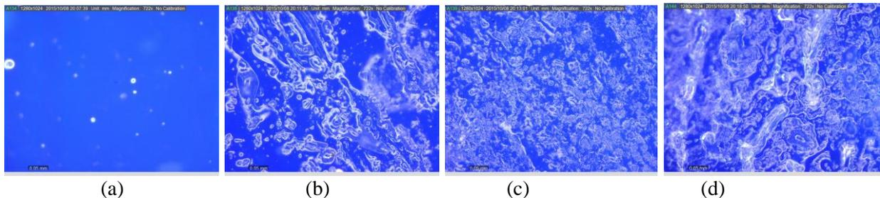
**Figure 8. Microscopic imaging of epoxy: (a) 0 week; (b) 2 weeks; (c) 4 weeks; (d) 6 weeks**
