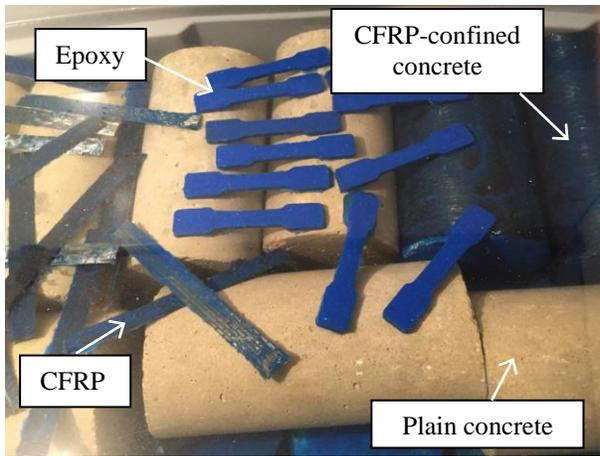
**Figure 1. Prepared specimens**
