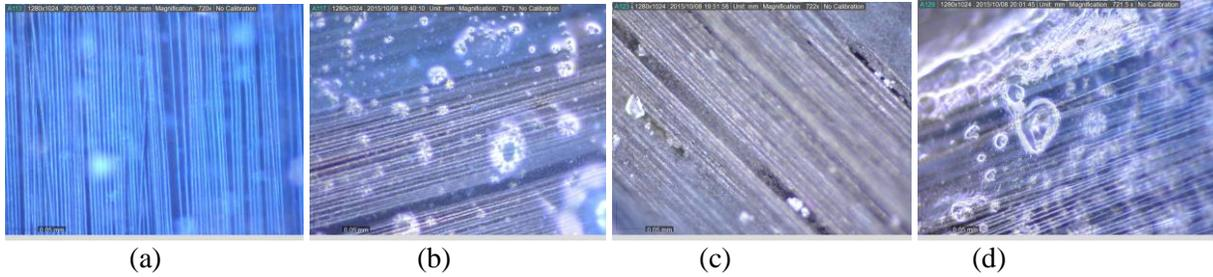
**Figure 9. Microscopic imaging of CFRP: (a) 0 week; (b) 2 weeks; (c) 4 weeks; (d) 6 weeks**
