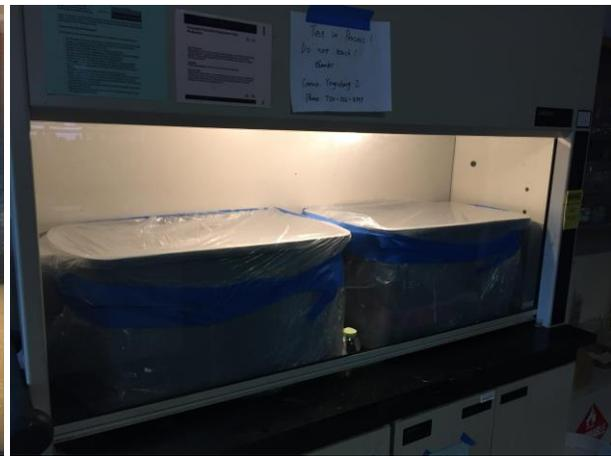
**Figure 2. Protected fume hood for conditioning**
