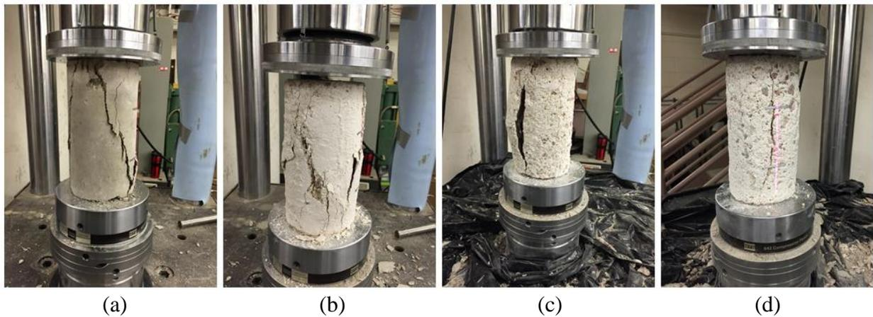
**Figure 11. Failure mode of plain concrete: (a) 0 week; (b) 2 weeks; (c) 4 weeks; (d) 6 weeks**
