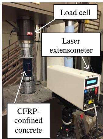
**Figure 5. Setup for cylinder testing**
