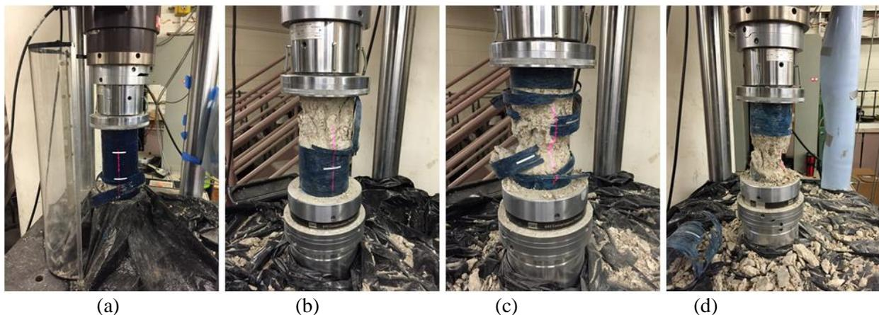
**Figure 12. Failure mode of CFRP-confined concrete: (a) 0 week; (b) 2 weeks; (c) 4 weeks; (d) 6 weeks**
