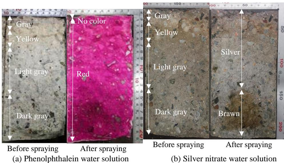
**Figure 13. Section of test specimen after heating and results from spraying phenolphthalein water solution or silver nitrate water solution**
