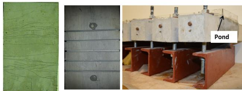
(b) Forming Cracks in FS31 specimens in flexural testing
