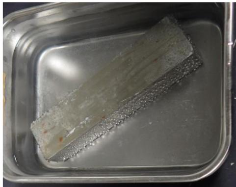
**Photo 11. Air pushed out from hardened cement paste**
