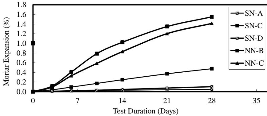
**Figure 1. Progression of mortar expansions obtained the study conducted by Islam (2010)**
