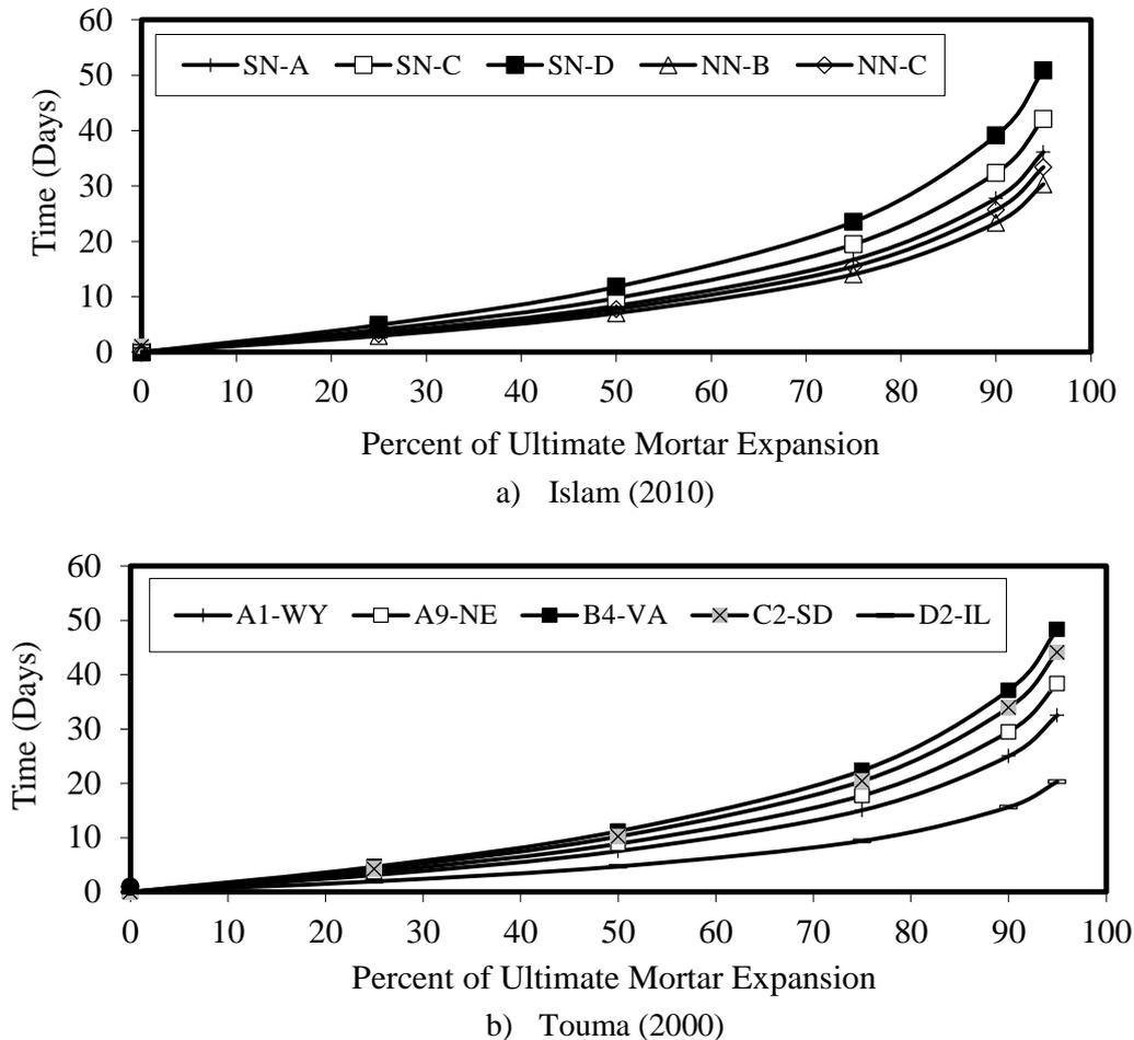
**Figure 2. Time required to reach percent of ultimate mortar expansion**
