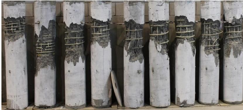
**Figure 3. Overview of the failure modes of GFRP RC columns**
