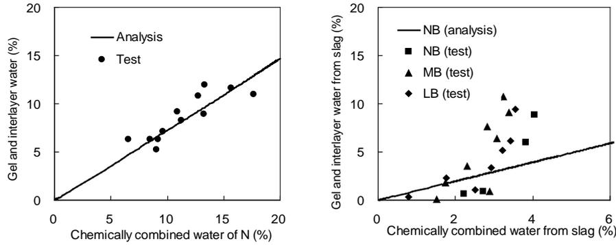
Fig. 6 Comparison of chemically combined water in hydrated pastes made with ordinary Portland cement (N) and BSF blended cements (NB, MB, LB).
