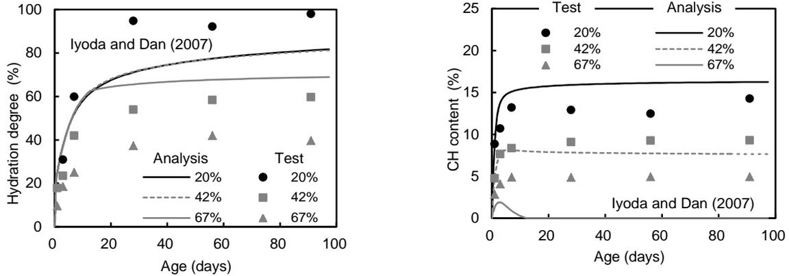
Fig. 9 Comparison of experimental data with value of original model analysis for hydration degree (left side) and CH content (right side)
