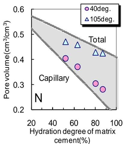
Fig.3 Relation between hydration degree of cement and pore volume.
