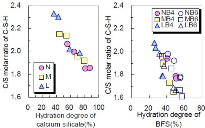
Fig.2 Ca/Si ratio of C-S-H in hydrated Portland and BSF blended cements
