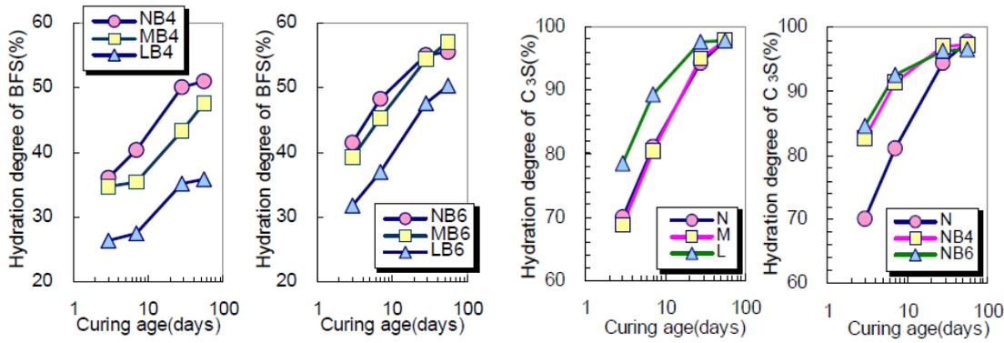
Fig.1 Degree of hydration of BFS and  $C_3S$  in BSF blended cement.
