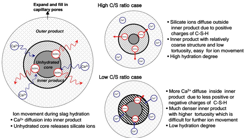
Fig. 10 Influence of inner product on ion movement and hydration of slag
