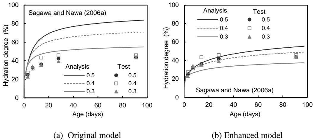
Fig. 11 Comparison of hydration degree based on enhanced model with original model: the water/binder ratios are 0.3, 0.4 and 0.5, slag replacement ratio is 50%, and slag powder with JIS fineness grade of 4000 is used.
