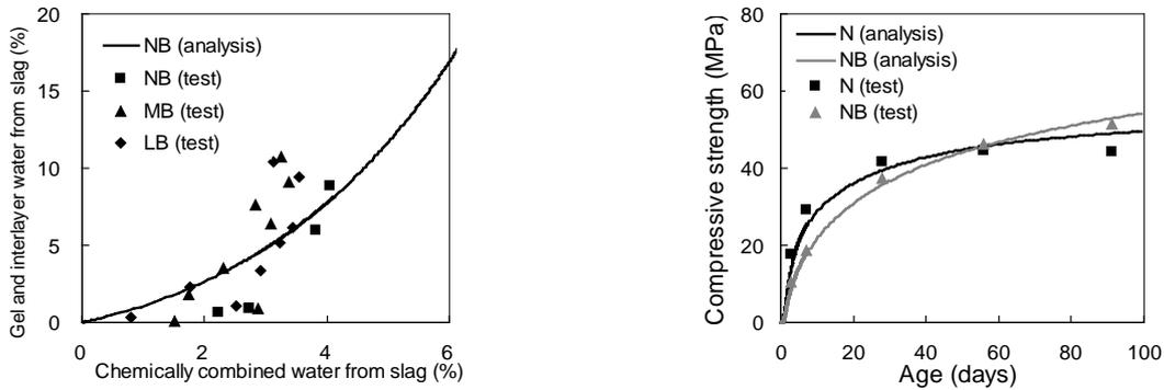
Fig.7 Gel and interlayer water in BSF blended cement paste (NB) based on enhanced model
