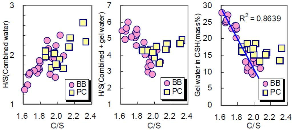
Fig.4 Chemical combined H<sub>2</sub>O to Si ratio (left), Chemical and gel and interlayer H<sub>2</sub>O to Si ratio (middle) and gel and interlayer water content in C-S-H represented as a function of Ca/Si ratio of C-S-H.
