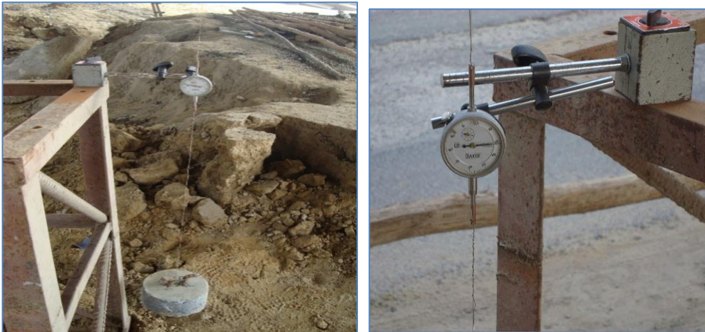
Figure 10. Typical arrangements for deflection measurement showing Dial gauge with suspended wire
