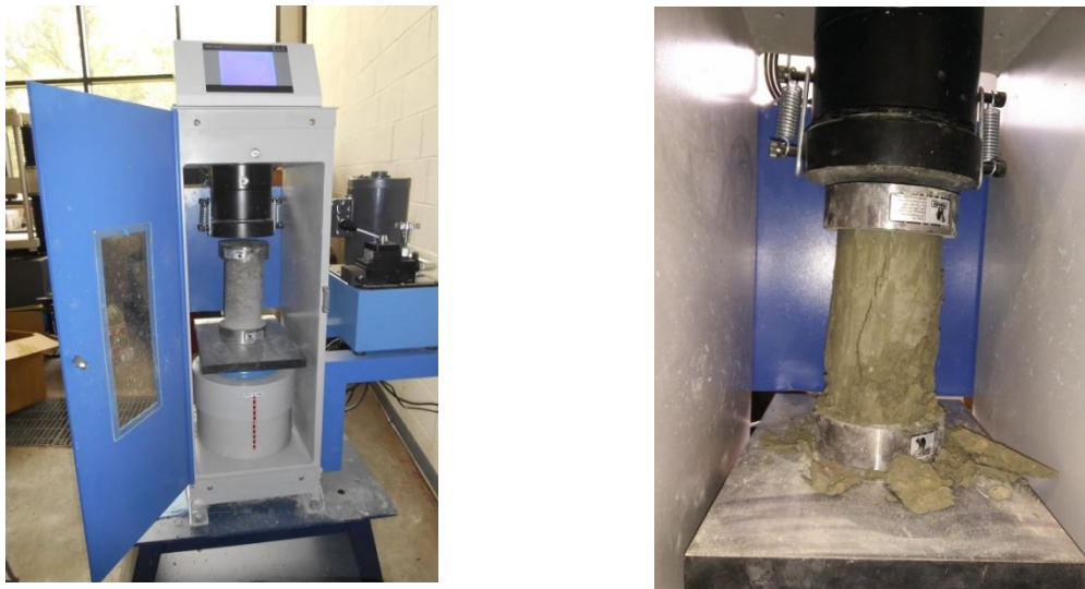
Figure 2. Compression Tester and 4-hour Compression Test
