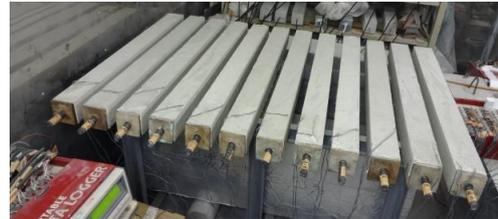
(b) Specimens stored in drying condition
