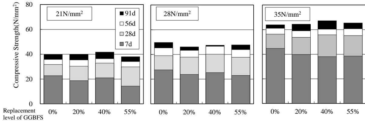
**Figure 2. Compressive Strength of Concrete**
