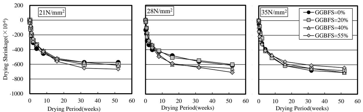
**Figure. 13 Drying Shrinkage of Concrete**
