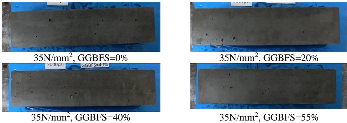
**Figure 6. Appearance of Concrete Specimens Submerged in Sulfate Solution (35N/mm<sup>2</sup>)**
