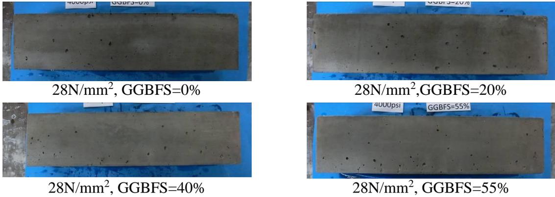
**Figure 5. Appearance of Concrete Specimens Submerged in Sulfate Solution (28N/mm<sup>2</sup>)**
