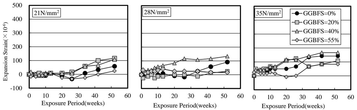
**Figure 3. Sulfate Expansion Strain of Concrete**
