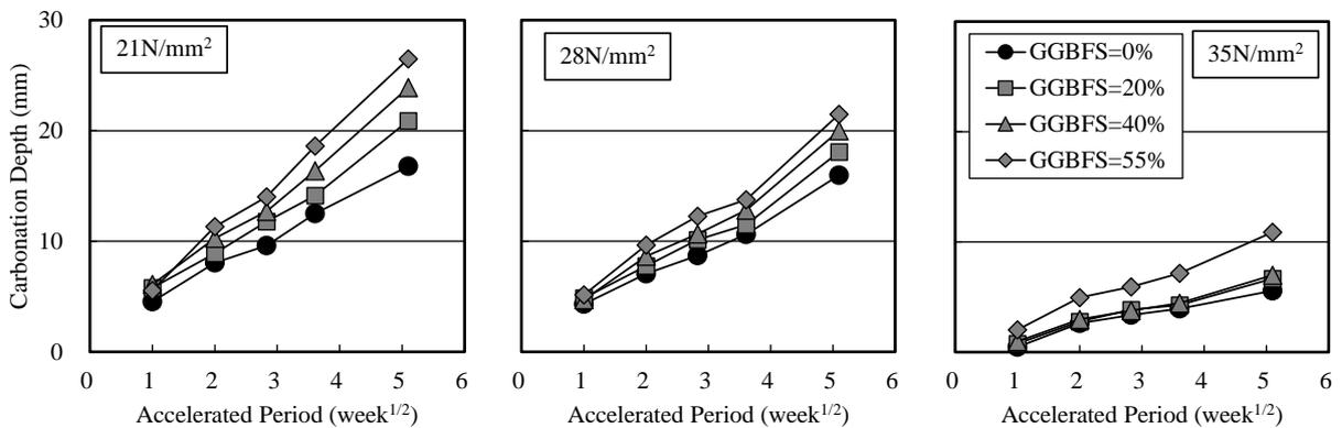
**Figure 7. Carbonation Depth of Concrete**
