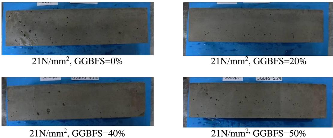
**Figure 4. Appearance of Concrete Specimens Submerged in Sulfate Solution (21N/mm²)**
