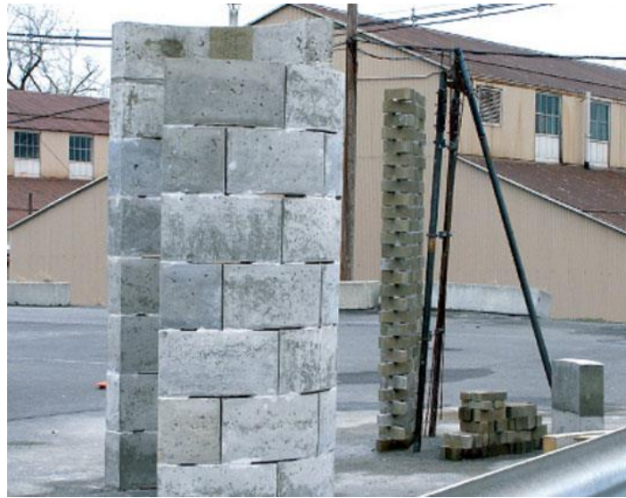
Figure 3. Building Bricks Containing Granulated Post Consumer Waste Plastics [ http://inhabitat.com/plastic-concrete-repurposes-landfill-waste-into-building-bricks ]
