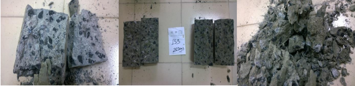
Figure 10. Fracture Surfaces of Concrete
