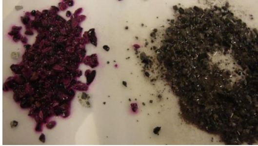
Figure 1. Carbonation tested by the solution of phenolphthalein (left: before carbonation; right: after carbonation)
