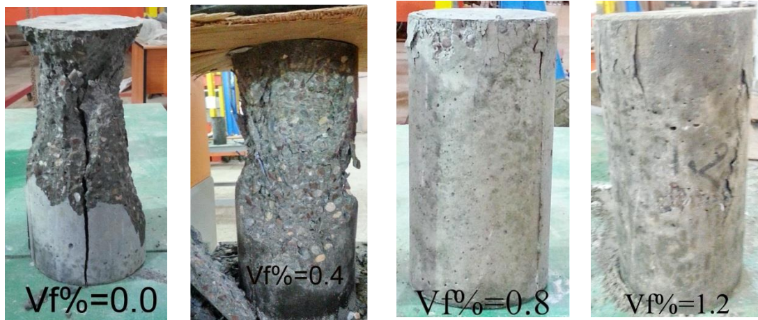
Figure 3. Typical Failed Compression specimens
