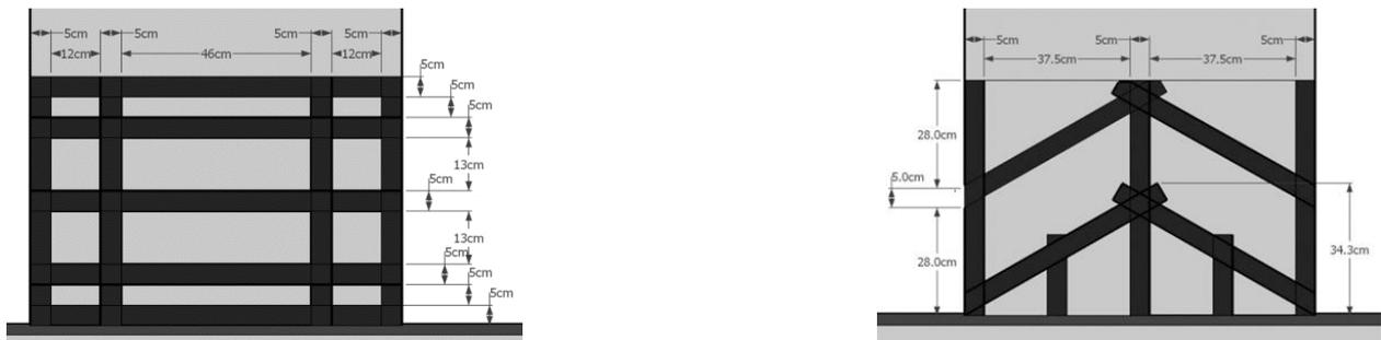
**Figure 2. CFRP reinforcement schematic detail (Wall SR4 and SR6)**
