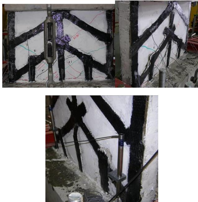
**Figure 5. Specimen SR6 Failure pattern**
