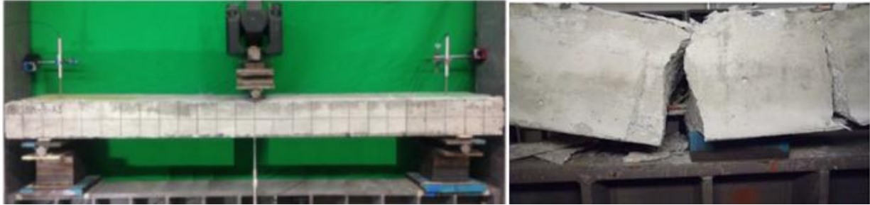
Figure 4. Fire-exposed Slab during Static Test and Failure Mode
