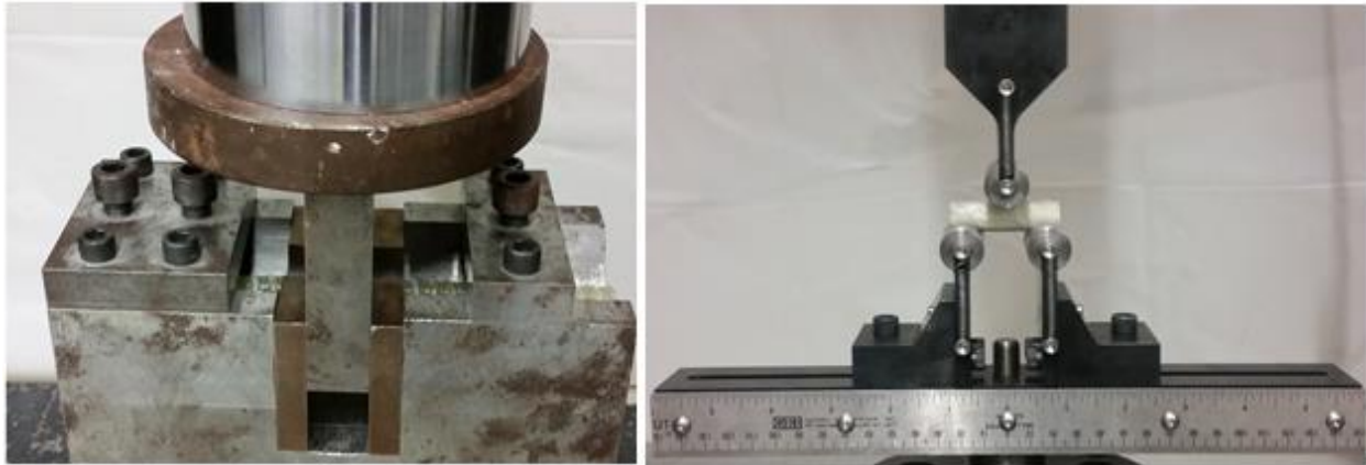
Figure 6. GFRP Bars Tested in Transverse Shear (left) and Short Beam Horizontal Shear (right)
