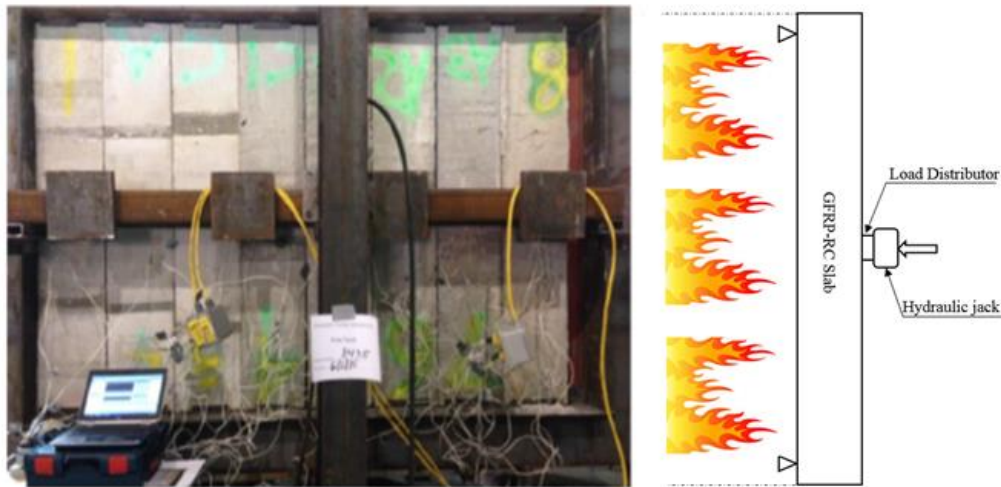
Figure 2. GFRP-RC Slabs during the Furnace Fire Test
