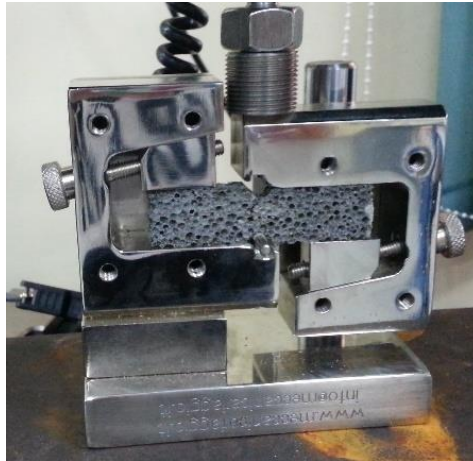
Figure 3. View of the complete setup for the shear test
