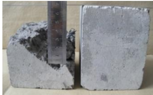
Figure 9. Determination of the spalling depth of specimen subjected to 800 °C
