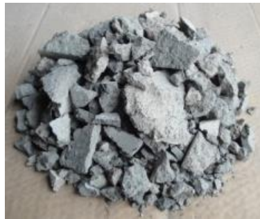
Figure 10. A severely spalled specimen
