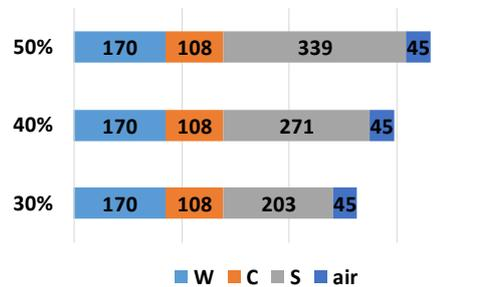
Figure. 2 Mix proportion of mortar
