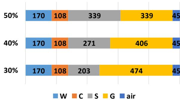
Figure. 1 Mix proportion of concrete
