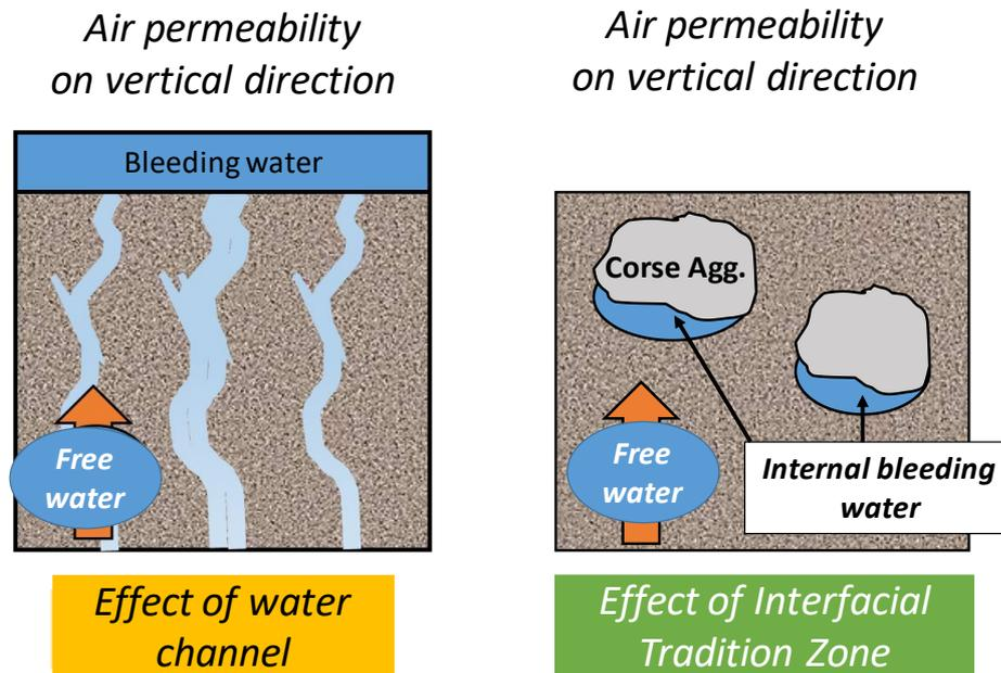
Figure. 6 Image of occurring gaps mechanism on different causes
