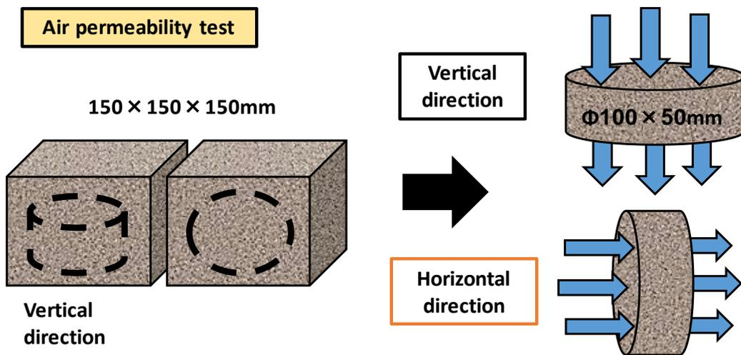
Figure. 3 Test flowchart
