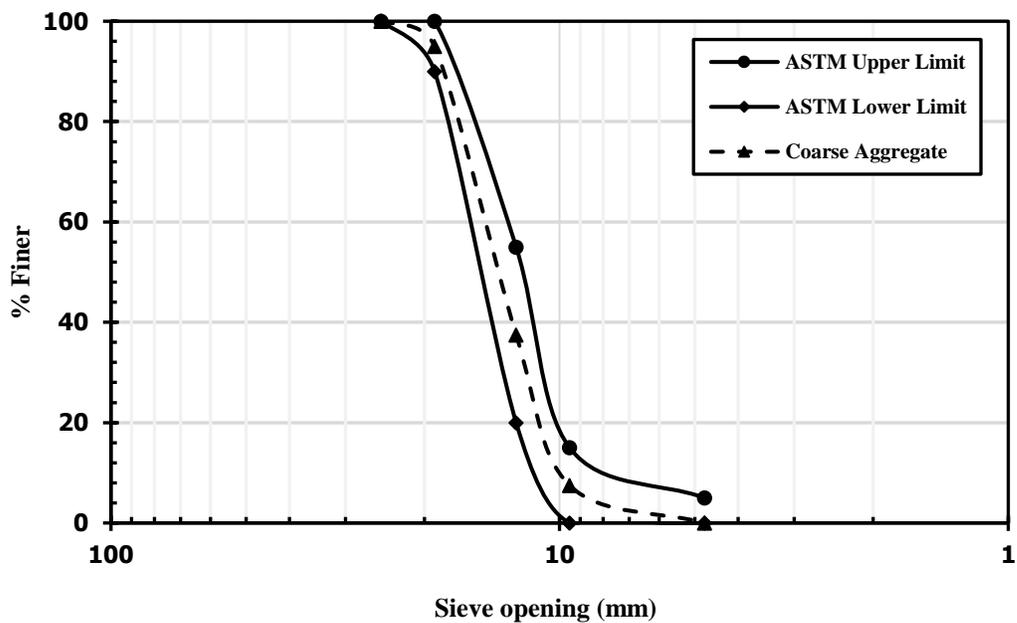
Fig. 2a. Gradation of coarse aggregate.
