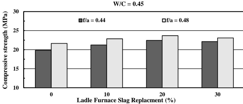
Fig. 6. Compressive strength of concrete made with 0% – 30% replacement ratios of LFS.
