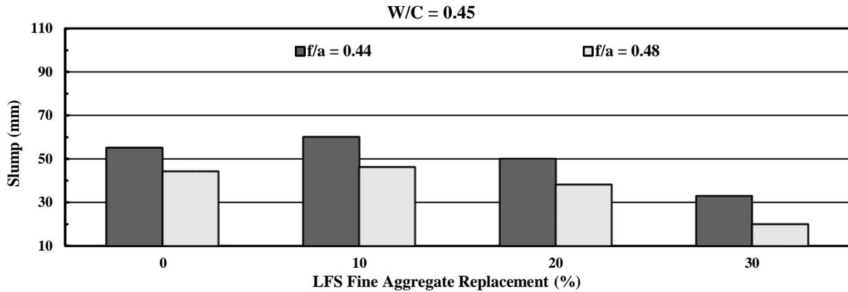
Fig. 4. Workability of concrete made with different replacement ratios of LFS.
