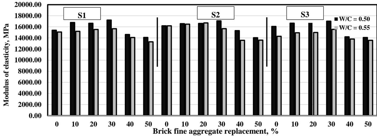
Fig. 7. 28-day tensile strength and modulus of elasticity of concretes made with BFA.
