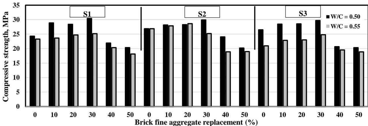
Fig. 5. Compressive strength of concrete made with 0% – 50% replacement ratios of BFA.
