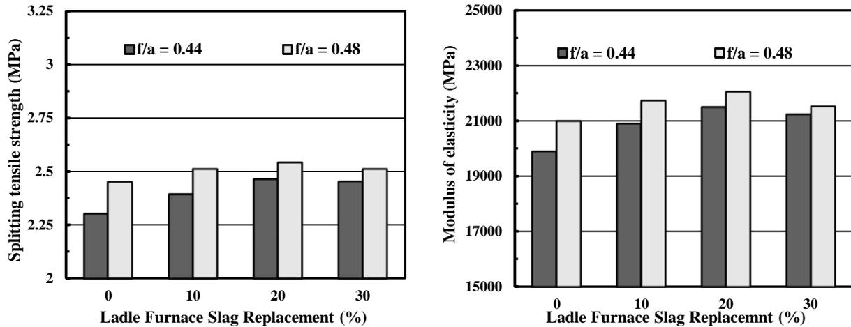
Fig. 8. 28-day tensile strength and modulus of elasticity of concretes made with LFS.
