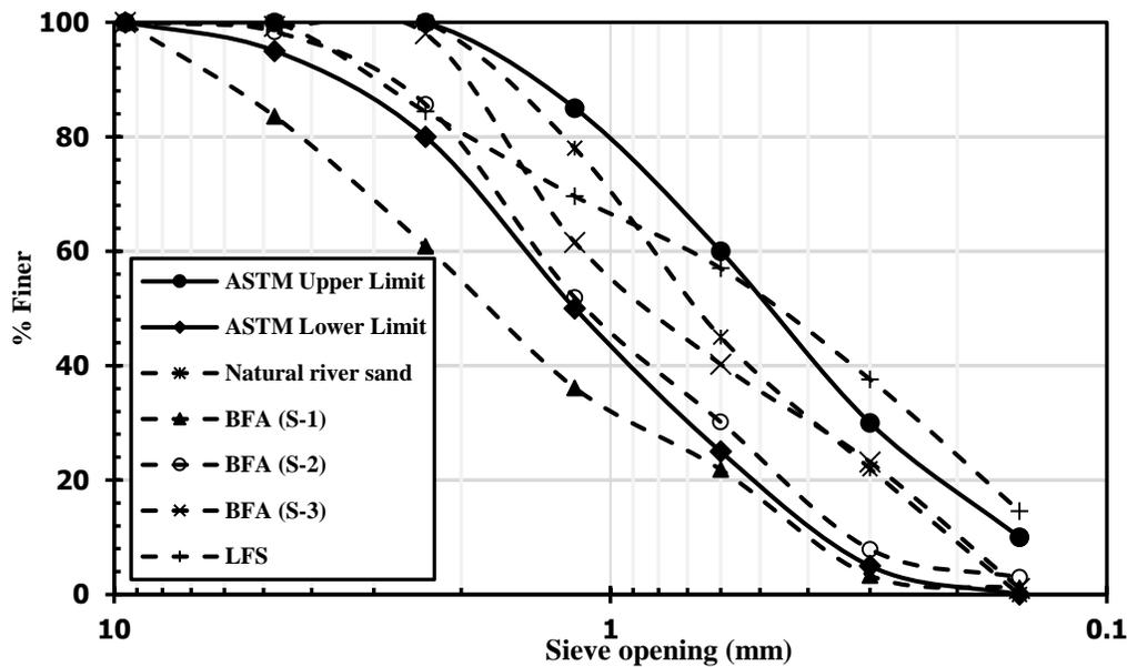
Fig. 2b. Gradation of fine aggregate.
