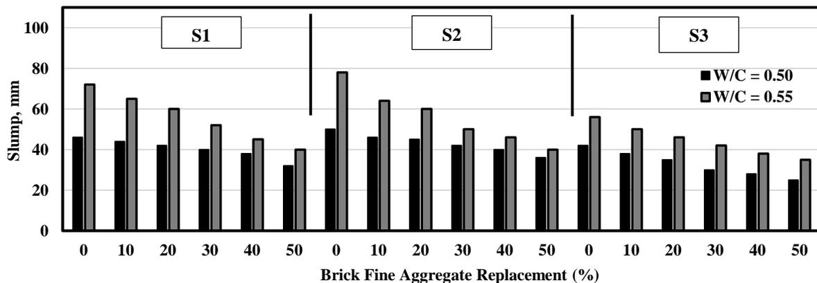
Fig. 3. Workability of concrete made with different replacement ratios of BFA.
