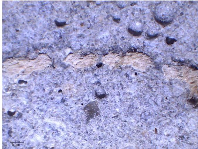
Figure 7. Detail of dense fique textile embedded into the mortar matrix
