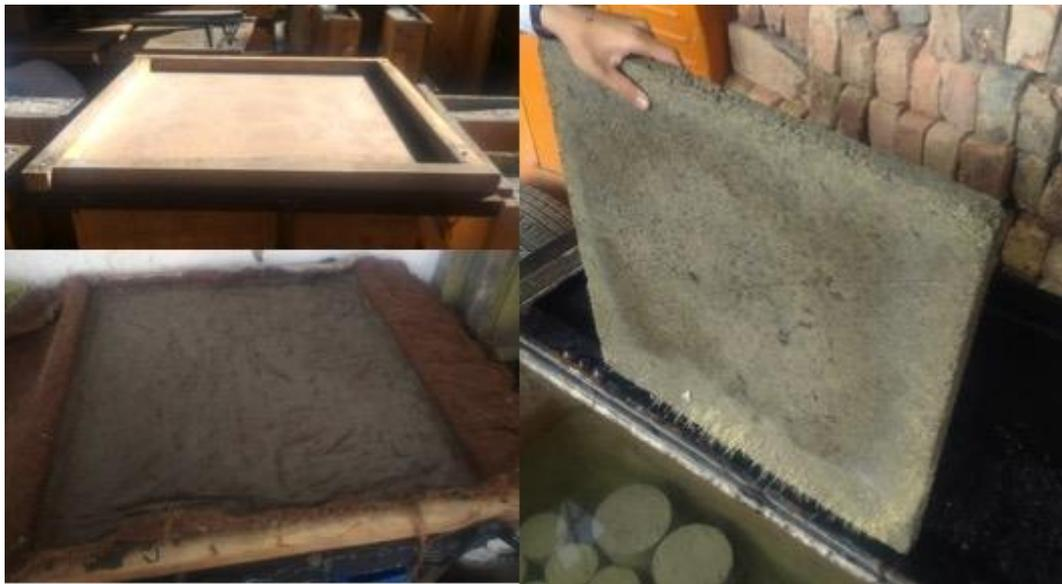
Figure 3. Fique composite manufacturing
