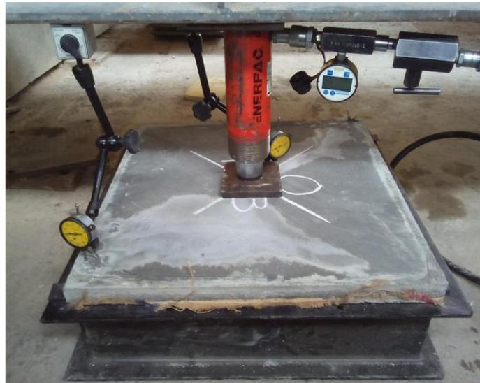
Figure 4. Experimental setup of the plate bending test
