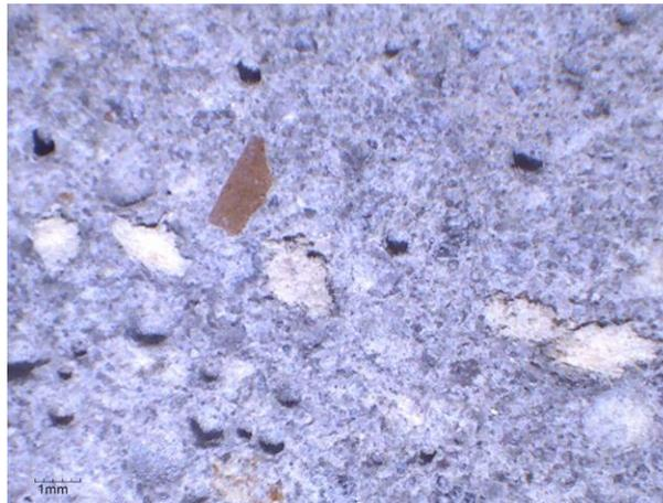
Figure 9. Detail of the standard fique textile embedded in the mortar matrix
