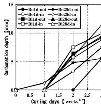
Fig.12 Carbonation depth and curing days
