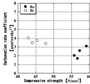
Fig.13 Carbonation rate coefficient and compressive strength
