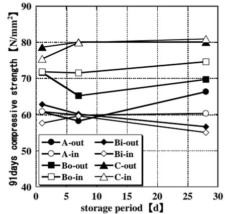
Fig.10 Compressive strength after 91 days
