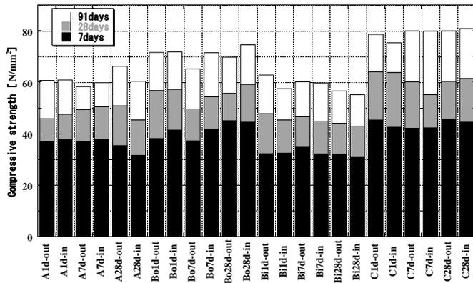
Fig.9 Compressive strength increased for all the FA types and storage conditions
