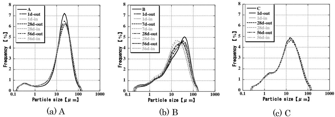
Fig. 2. The particle size distribution
