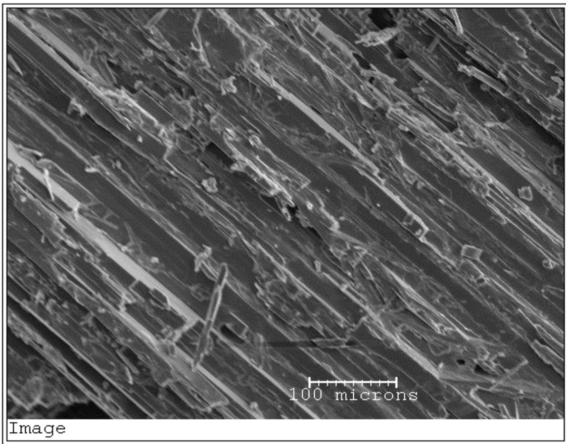
**Figure 2:** Secondary electron image of fracture surface of unhydrated slag.
