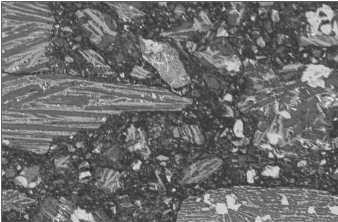
**Figure 4:** Backscattered electron image of polished surface of the hydrated spent borax paste (same scale as Figure 2). The white area is metal-substituted metallic oxide, the light grey area is metallic oxide, the dark grey area is sodium tetraborate oxide and the black area is fracture porosity.
