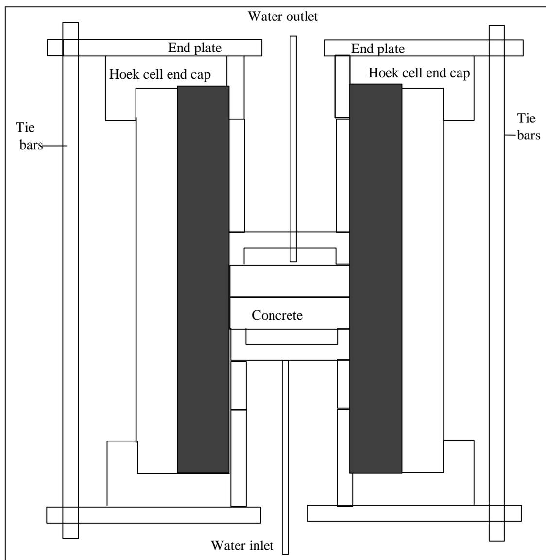
**Figure 5:** Schematic view of high-pressure cell
