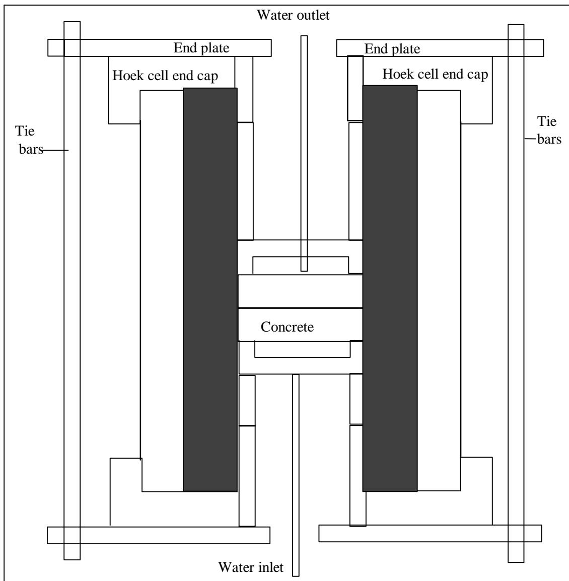
**Figure 5:** Schematic view of high-pressure cell
