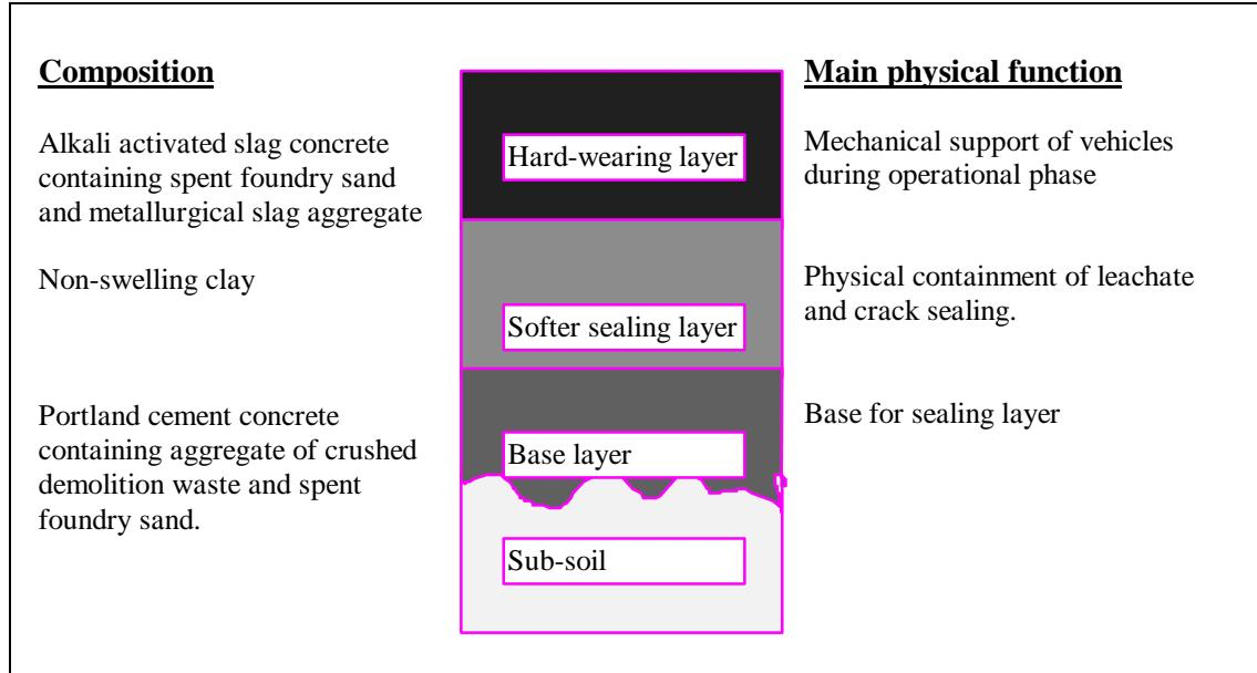
**Figure 1:** Schematic cross-section of composite landfill liner.
