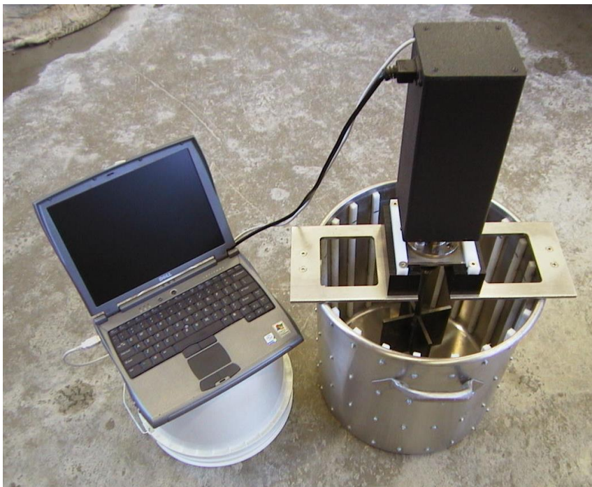
Figure 4.7: Assembled ICAR Rheometer (Germann Instruments 2007)
