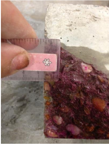
Fig 5.41 Binder Mix Concrete Sample (0.5 W/B) Dry Cured – 3.5mm Carbonation
