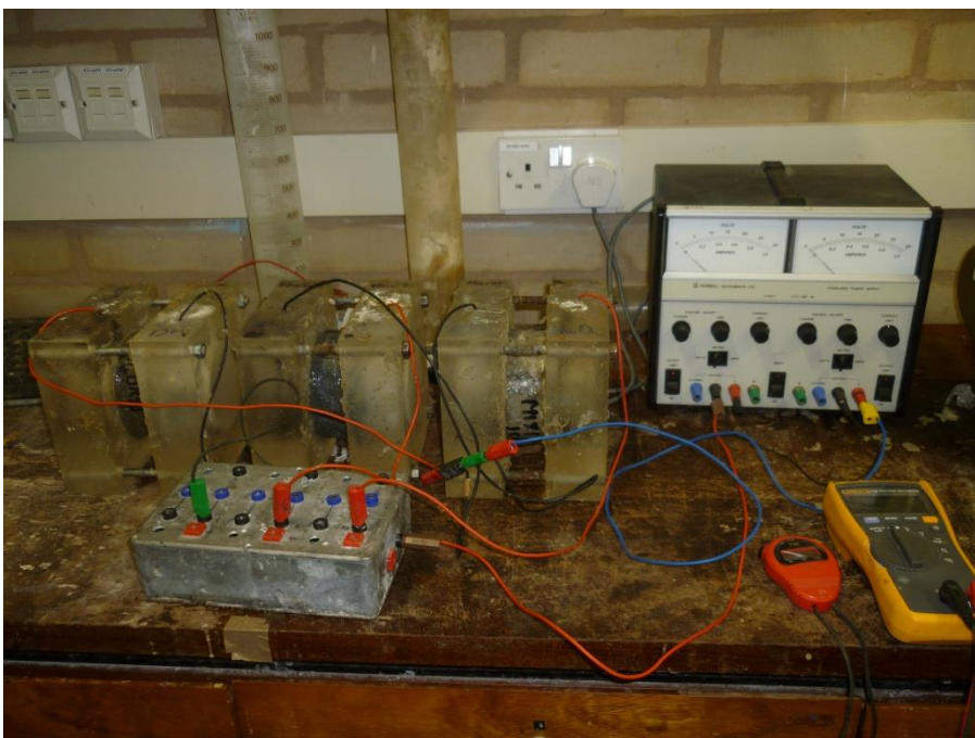
Figure 4.24: RCPT test setup
