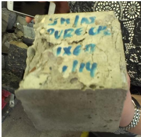
Figure 5.23: compressive strength failure pure OPC
