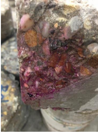
Fig 5.45 Binder Mix Concrete Sample (0.6 W/B) Wet Cured - 7mm Carbonation
