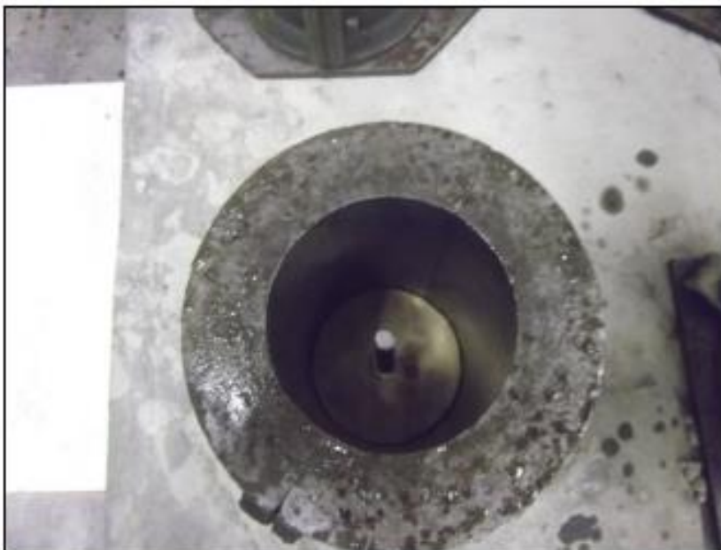
Figure 4.25: Shows the moulds used to cast the cylinders - (Proctor 2012)
