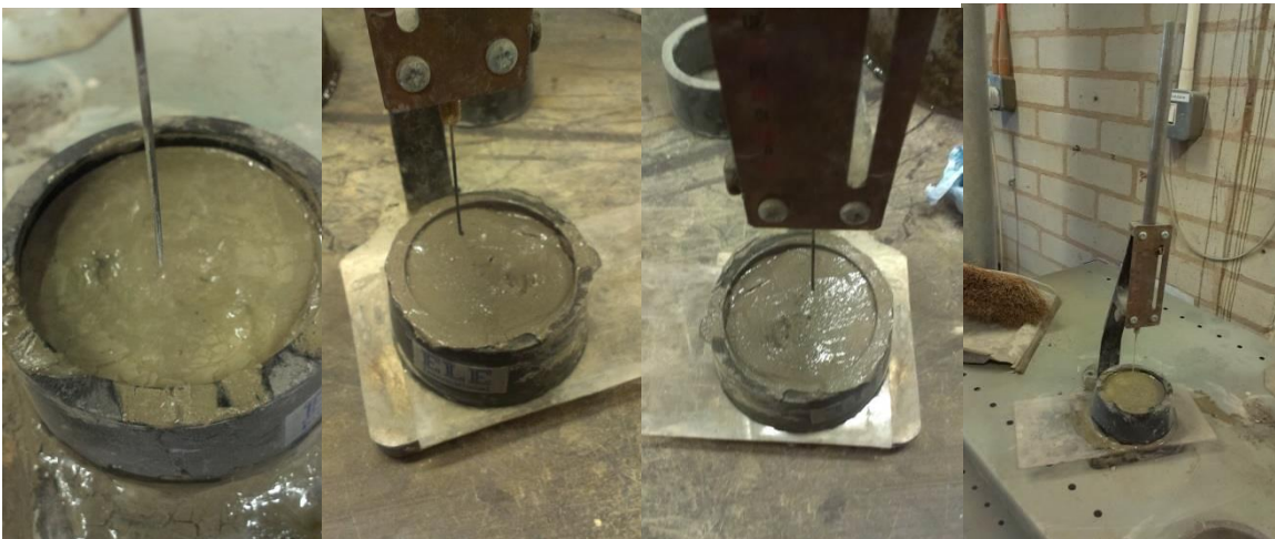
Figure 5.57: The testing of the samples and the Vicat needle apparatus
