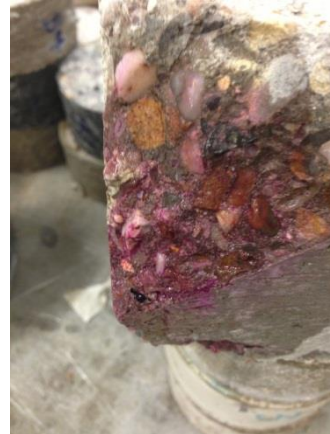
Fig 5.46 Binder Mix Concrete Sample (0.6 W/B) Dry Cured - 4mm Carbonation
