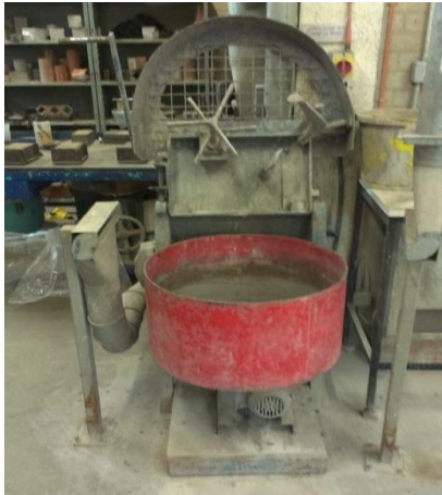
Figure 4.1: Median mixer used for mixing the test samples of Setting Time and Heat of Hydration
