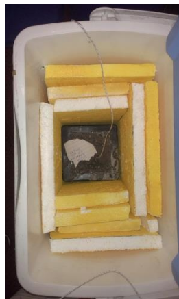
Figure 4.42: Heat of Hydration insulated boxes
