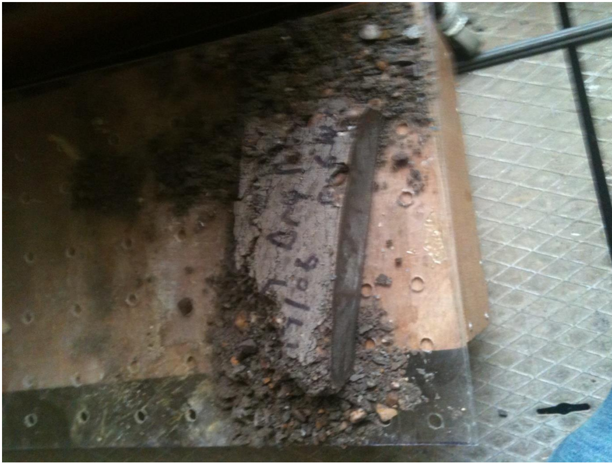
Figure 4.16: Failed Binder Mix 8 Sample
