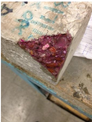
Fig 5.37 Pure OPC Mix Concrete Sample (0.5 W/B) Wet Cured - 0mm Carbonation
