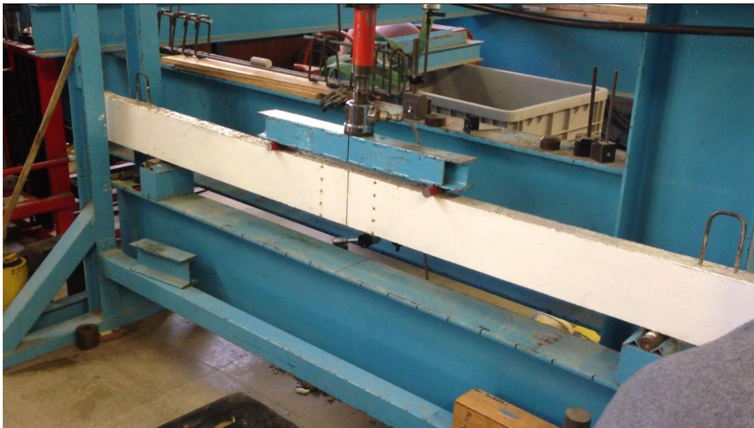
Figure 4.29 Structural Loading of Beam
