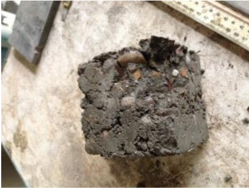
Figure 4.40: Actual Sample Taken Post Compressive Strength Test
