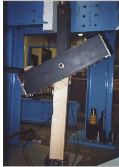
*Figure 4.28 Sample configuration for tension test with load at  $60^\circ$  to the grain.*
