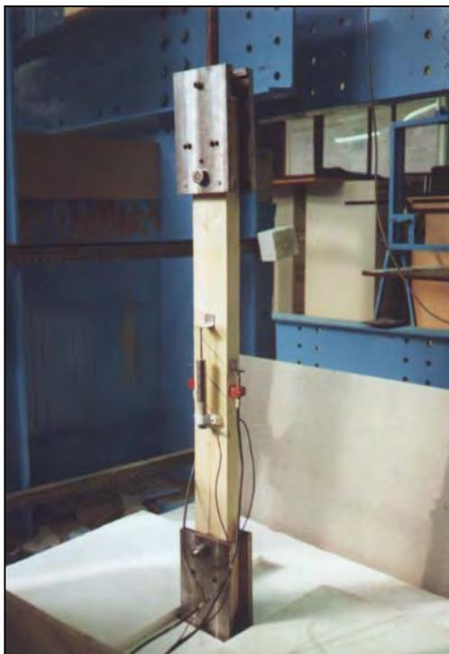
*Figure 4.22 TPB00 sample ready for straight pullout test.*
