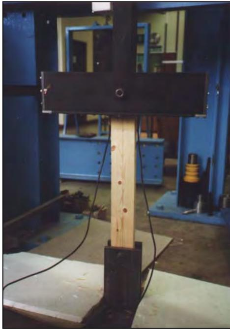
*Figure 4.27 Sample configuration for tension test with load at  $90^\circ$  to the grain.*
