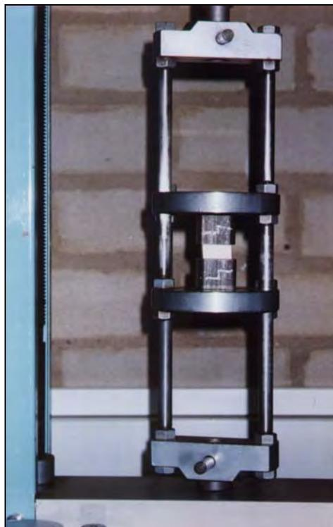
*Figure 4.63 Shear parallel to the grain test configuration.*
