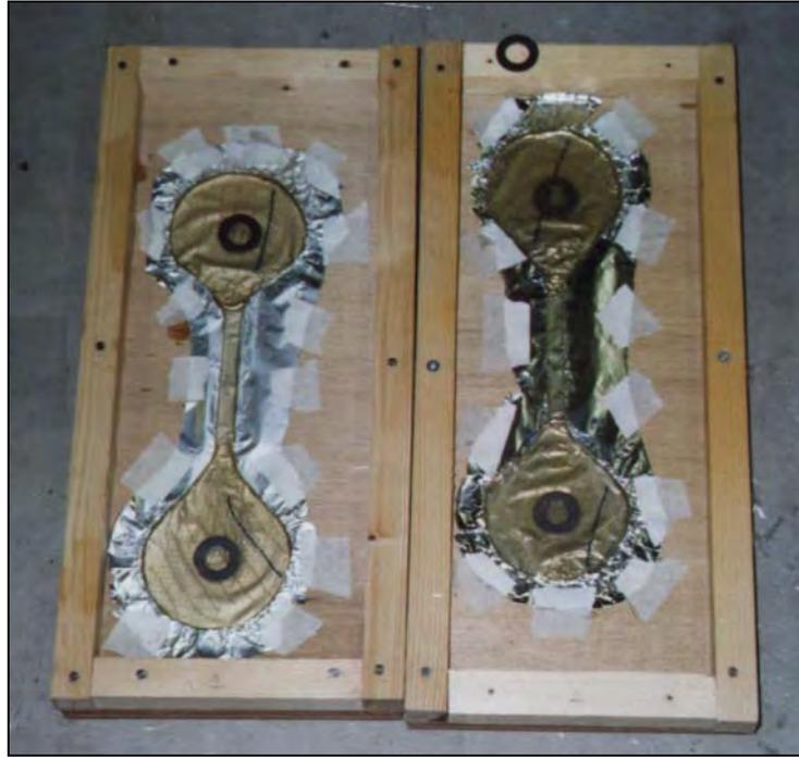
*Figure 4.3 Dog bone samples curing in moulds.*
