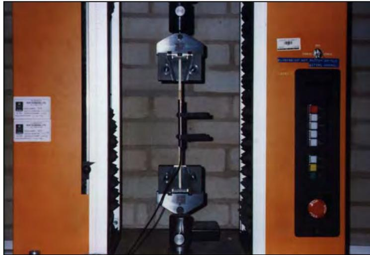
*Figure 4.54 Tension parallel to the grain test configuration.*
