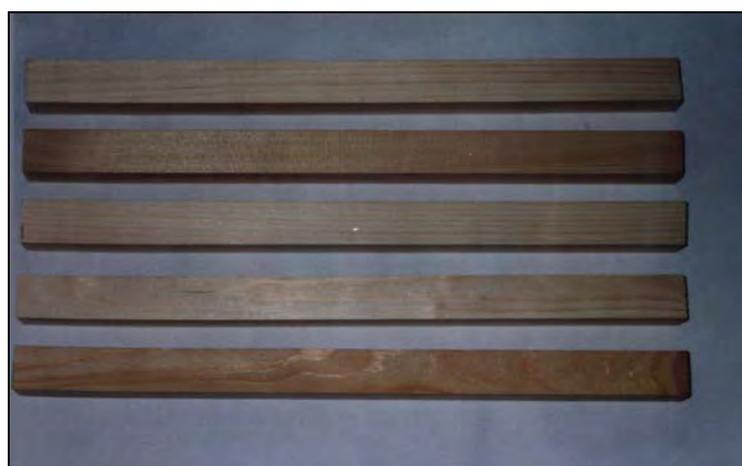
*Figure 4.49 Static bending test samples.*
