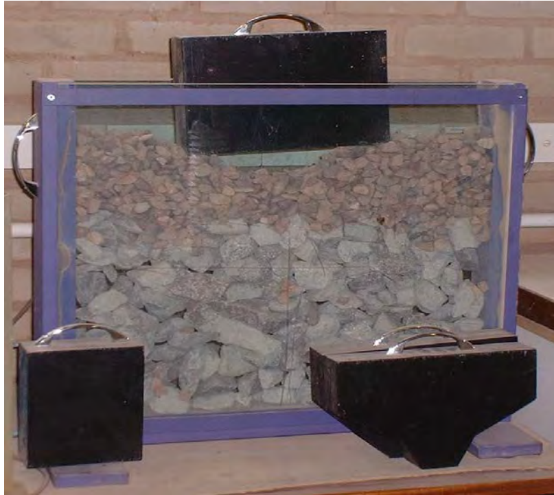
Figure 4.1 Two dimensional representation of track ballast and sleepers
