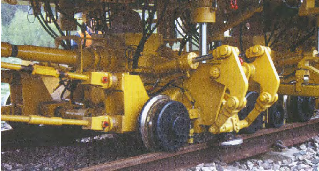
Figure 2.42 Close-up view of dynamic track stabilizer unit (Cope and Ellis 2001)
