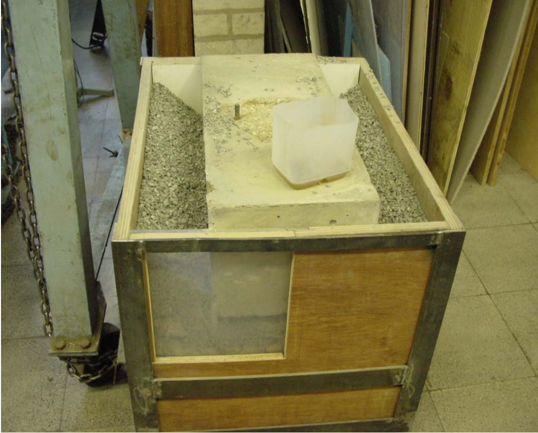
Figure 6.7a Test with 5mm crib ballast - photograph taken after the test was complete.
