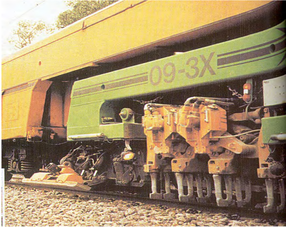
Figure 2.26 A close up view of on track tamping machine showing the tamping tines.
