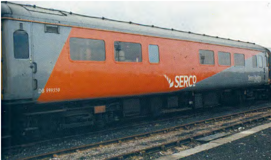
Figure 2.21 High speed track recording car capable of recording at speeds of 125miles per hour (Cope and Ellis 2001)
