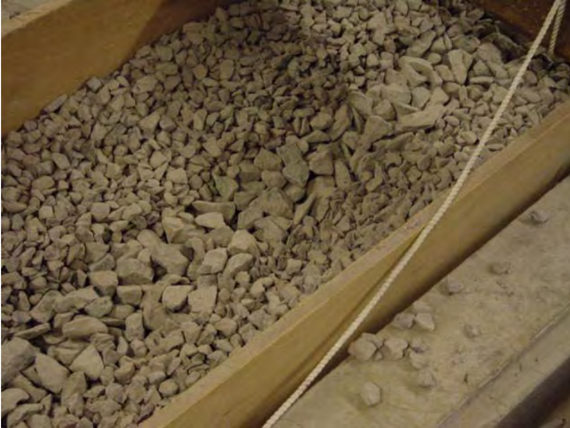
Figure 6.11b Movement of crib ballast below the sleeper
