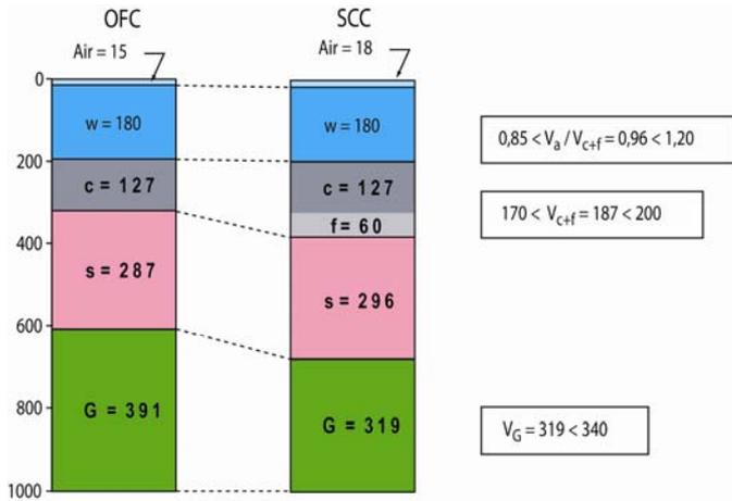
Figure 2. Composition in volume ( $L/m^3$ ) of the ingredients in the Ordinary Concrete (OC) and SCC.
