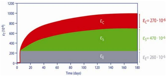
Figure 11. OFC: elastic strain ( $\epsilon_E$ ), drying-shrinkage ( $\epsilon_S$ ) and creep strain ( $\epsilon_C$ ) at R.H. of 65% with a load of 170 MPa at 7 days (1/4 of 68 MPa).
