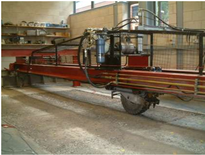
Figure 6 Trafficking trial pavement in the PTF
