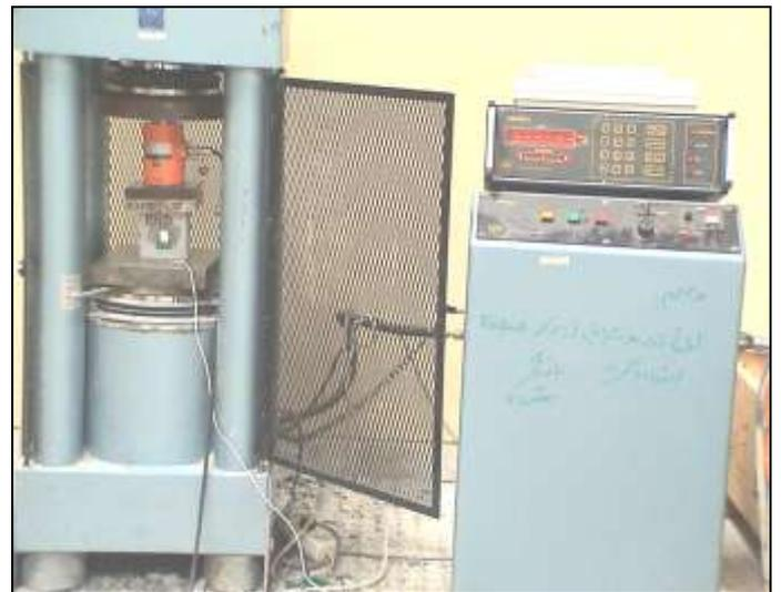
Figure 9. Uniaxial compressive test
