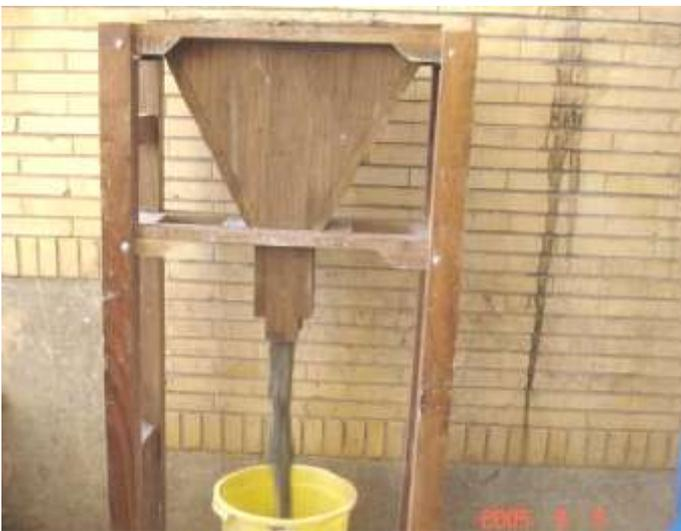
Figure 4. V-funnel test of SCLC
