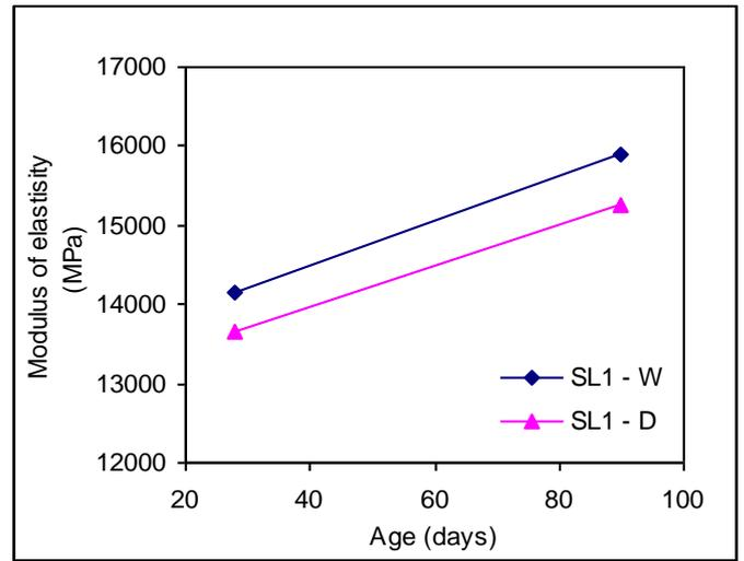
Figure 16. Modulus of elasticity of SL1 in (W) and (D) conditions
