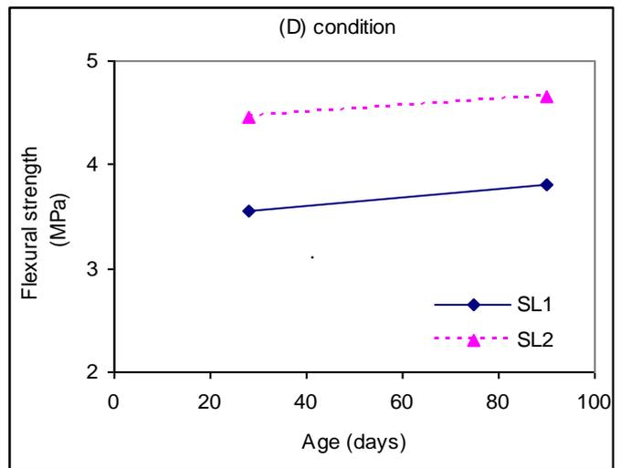
Figure 13. Flexural strength of SL1 and SL2 in (D) condition
