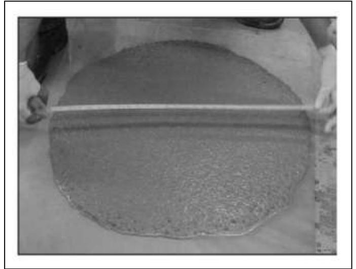
Figure 2. Slump flow test of SCLC
