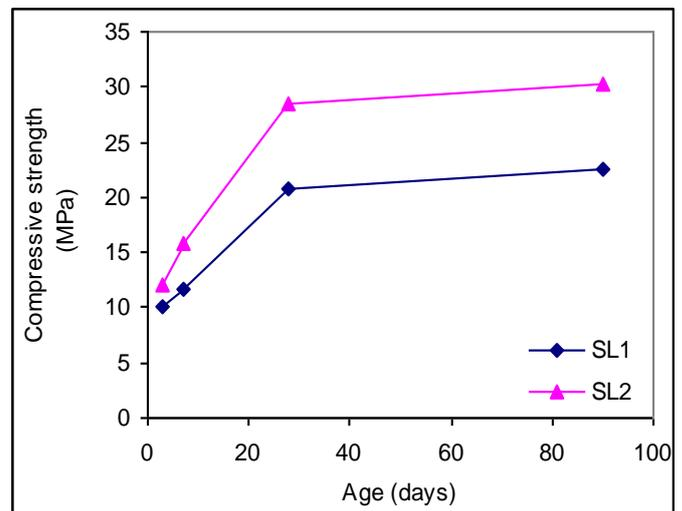
Figure 6. Compressive strength of SL1, SL2 in (W) condition
