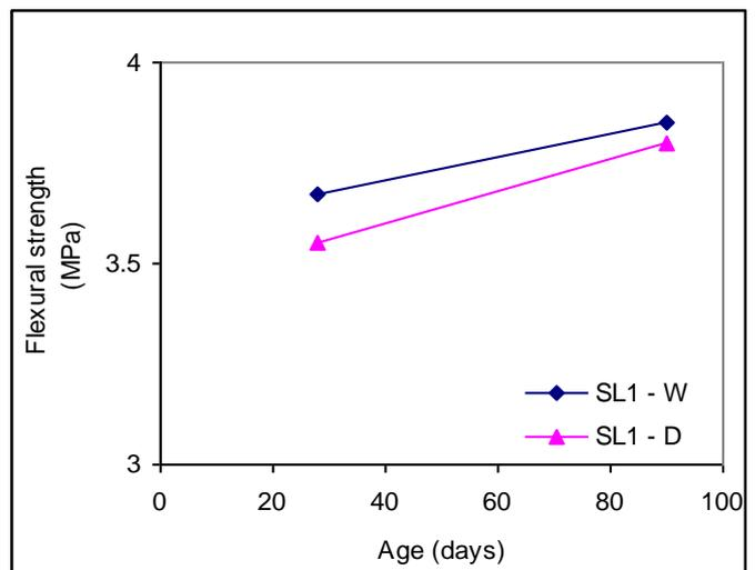
Figure 14. Flexural strength of SL1 in (W) and (D) conditions
