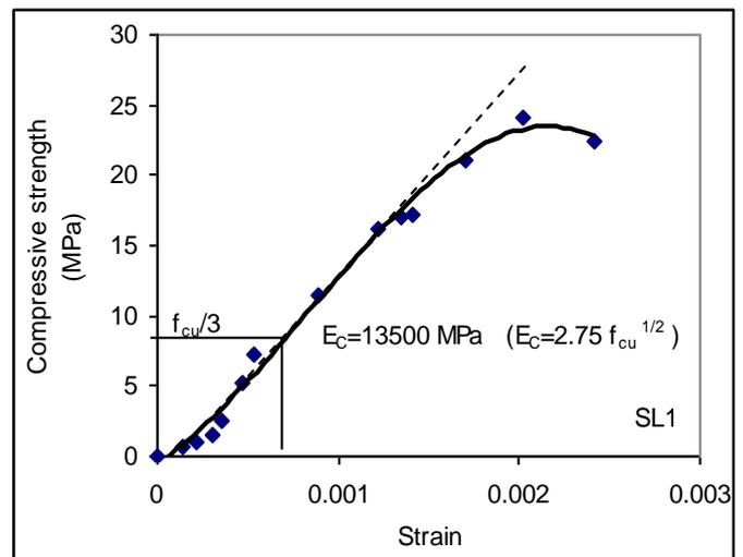
Figure 10. Stress-strain curve for SL1
