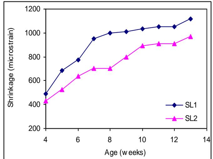
Figure 18. Shrinkage of SL1 and SL2 in (W) condition
