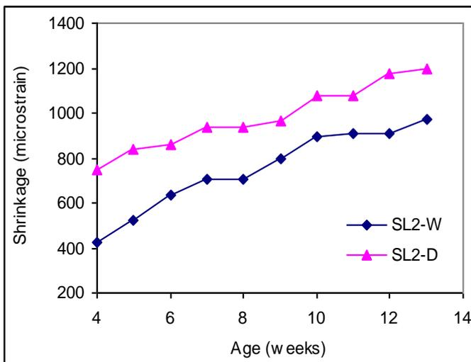
Figure 21. Shrinkage of SL2 in (W) and (D) conditions
