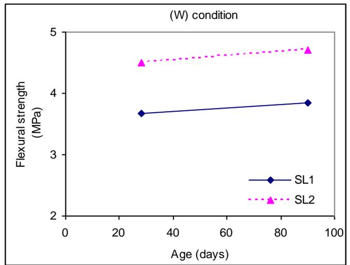
Figure 12. Flexural strength of SL1 and SL2 in (W) condition
