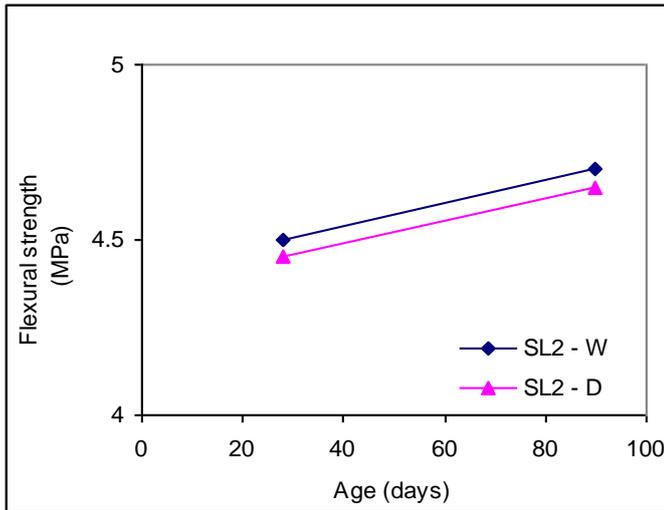
Figure 15. Flexural strength of SL2 in (W) and (D) conditions
