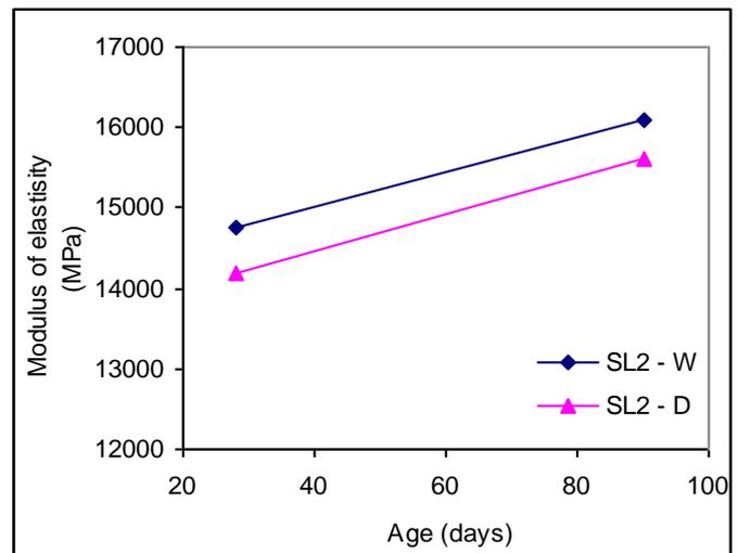
Figure 17. Modulus of elasticity of SL2 in (W) and (D) conditions
