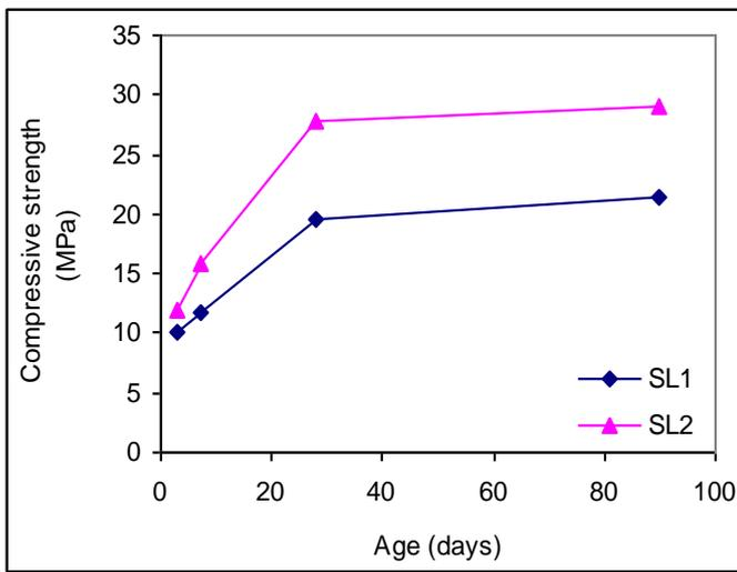
Figure 7. Compressive strength of SL1 and SL2 in (D) condition
