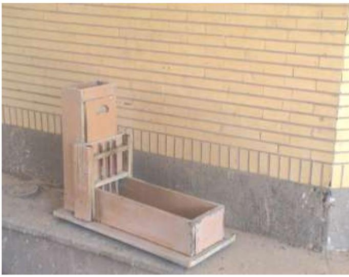
Figure 5. L-box test of SCLC
