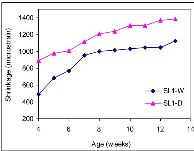
Figure 20. Shrinkage of SL1 in (W) and (D) conditions
