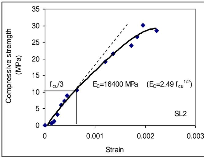
Figure 11. Stress-strain curve for SL2
