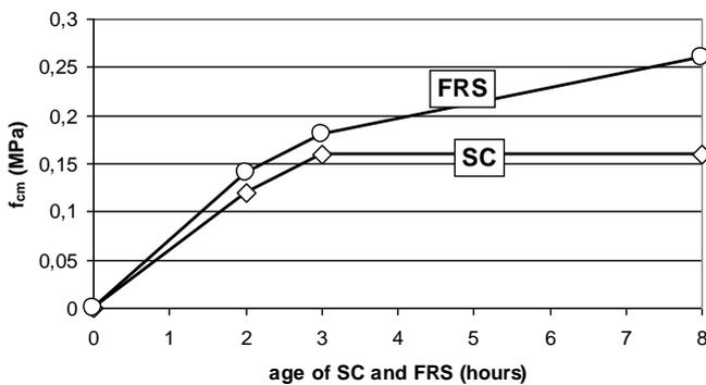
Figure 7: Average values of peak stress  $f_{cm}$  of SC and FRS at ages of 2, 3 and 8 hours.
