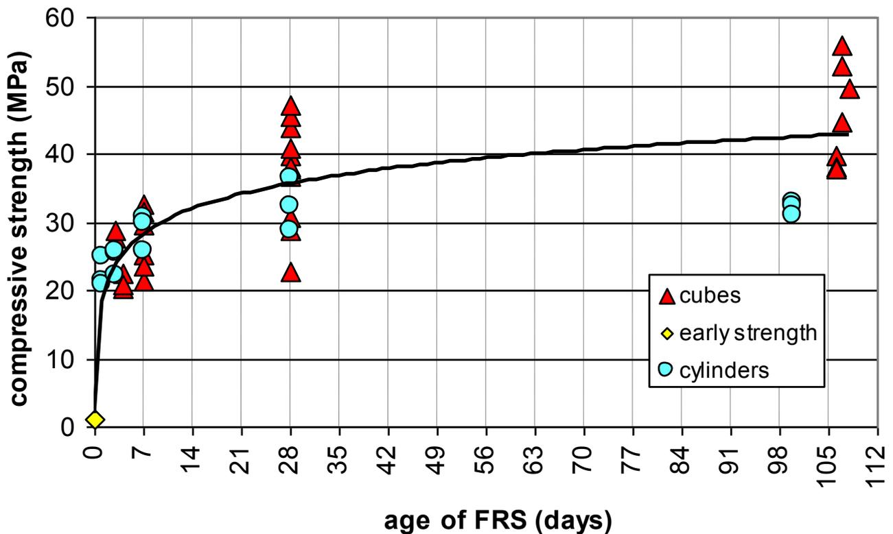
Figure 1. Influence of age of FRS on compressive strengths.
