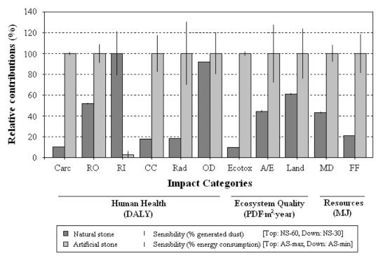
Figure 4. Comparative characterisation with sensibility analysis (Eco-Indicator 99).
